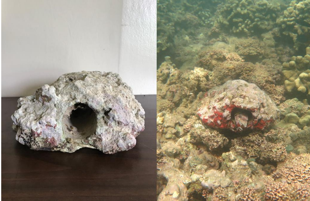
Figure 8. Artificial rock used to deploy temperature loggers at the Kualoa and Kailua study sites (left), and an example photograph of a temperature logger inside the rock on the reef flat (right).
