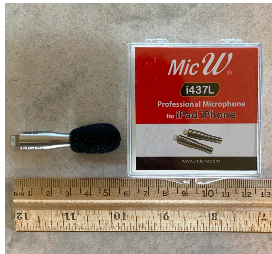
(d) MicW i437L Omnidirectional Measurement Microphone (Lightning Connector) with a frequency band from 20 Hz to 20 kHz, sensitivity of -27.5 dBFS (94dB SPL at 1 kHz), a signal-to-noise ratio over 62 dB, connects directly to iPhone or iPad via light, and weighs 10 g (User's manual)
