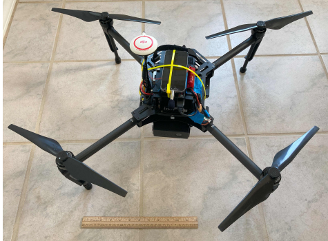
(a) The DJI M100 (2015) has arms of length \ell = 0.31 m, 13" propellers with pitch of 4.5", and a total mass of m = 3.133 kg with one TB48D 6S (5700 mAhr) battery
