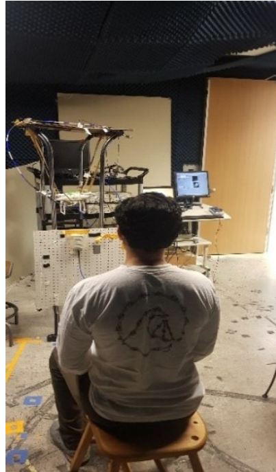
Fig 6.2: Setup for experiment inside an anechoic chamber. A subject sitting comfortably in front of doppler radar facing front at 1.1 m distance from radar
