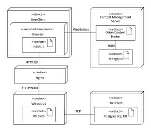
Figure 7. FIWARE Orion offering a WebSocket-Port to avoid the CORS problem
