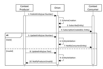
Figure 5. Sequence Diagram of a centralized schema validation through Orion
