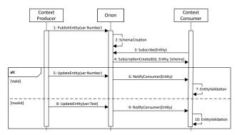
Figure 6. Sequence Diagramm example of how Orion could provide schemas for a entity validation through context consumers
