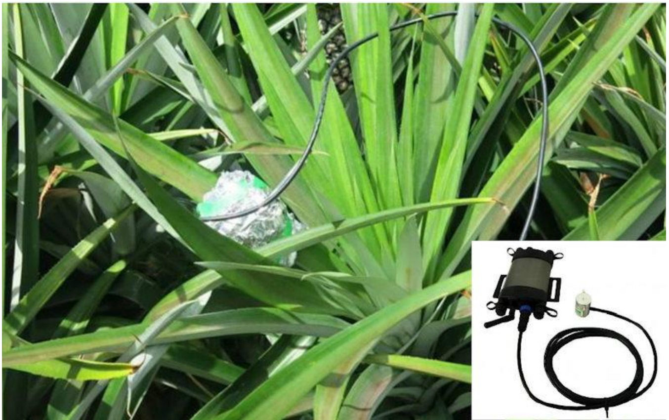
Figure 2. Pineapple plant with the insulated psychrometer (PSY1) installed in the leaf (Inset: PSY1 instrument).
