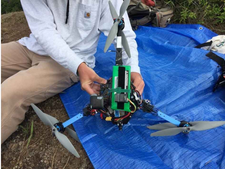
Figure 12. Y-6 rotary UAS being prepped for launch.
