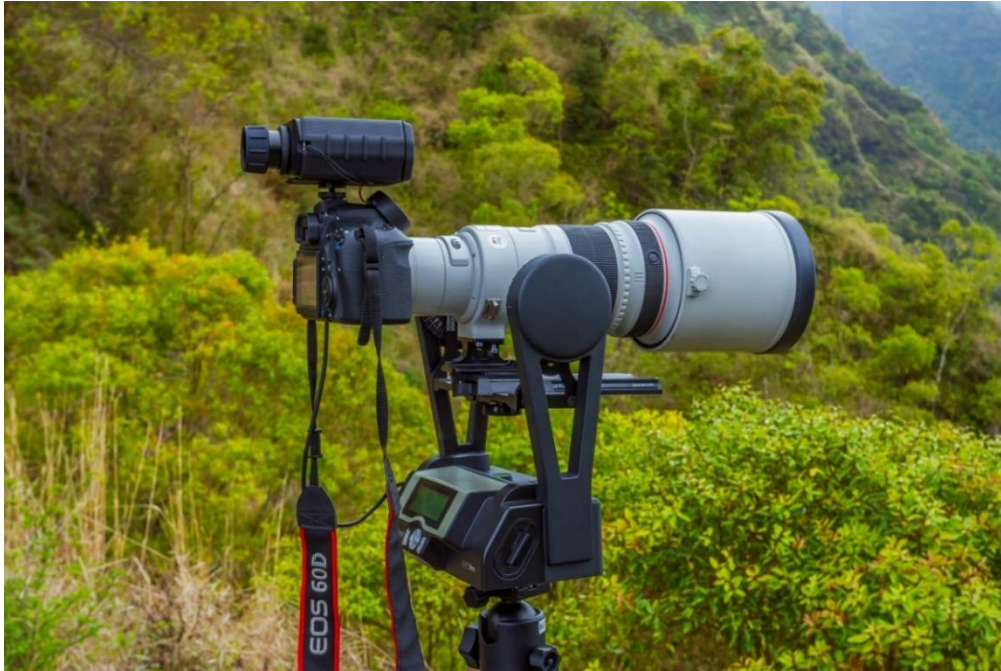
Plate 1. Tested Gigapan®, camera and lens configuration with Truepulse® laser rangefinder.
