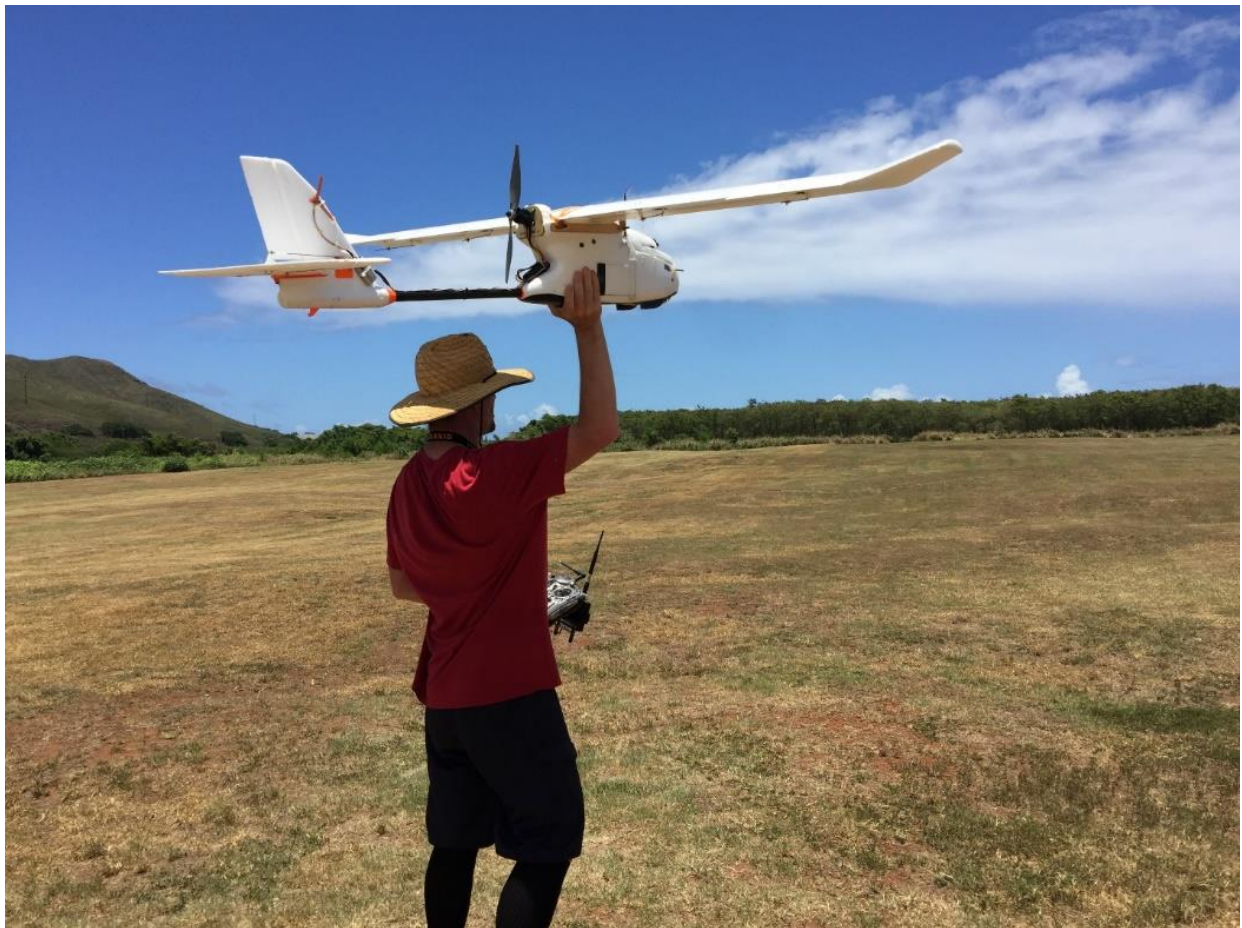
Figure 14. Skywalker 1900 fixed wing UAS pre-launch for test flight by Charles Devaney.
