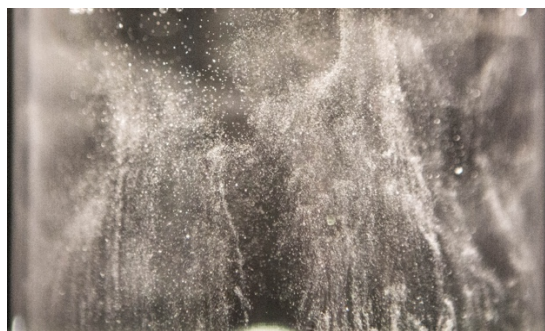
Figure 24. Microbubbles produced by TiPt electrodes during EF.
