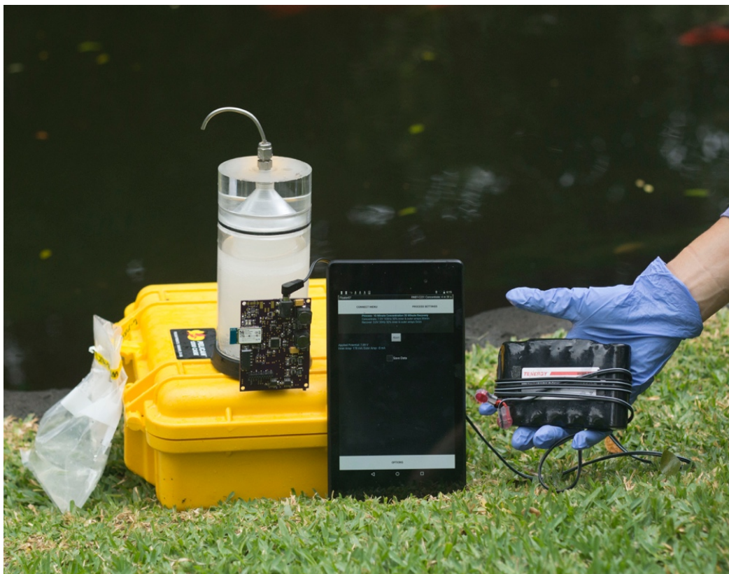
Figure 35. Image of Electroflotation System. For testing the efficacy of electroflotation treatment for point-of-care sample preparation we designed a self-contained battery powered EF cartridge interfaced wirelessly to an Android app.
