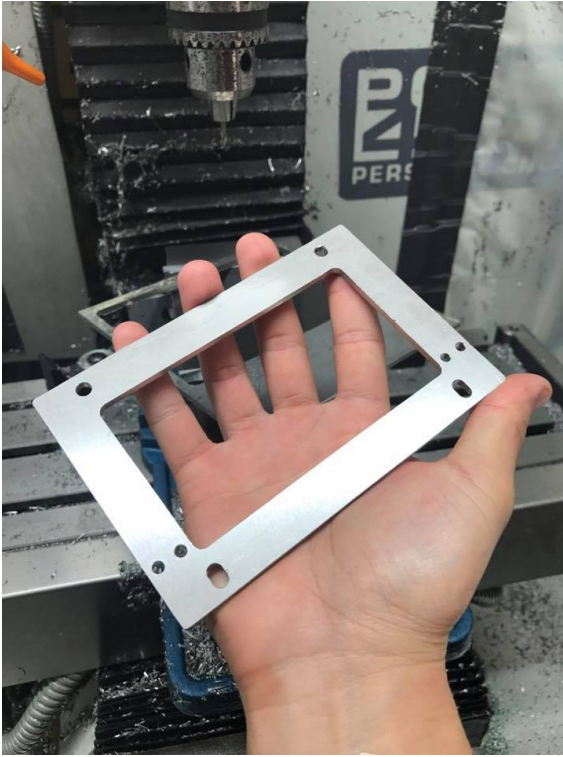
Figure 64: The finished machined 17-5 PH. Machine time was about 2 hours using a 1/8" 5 flute carbide endmill.
