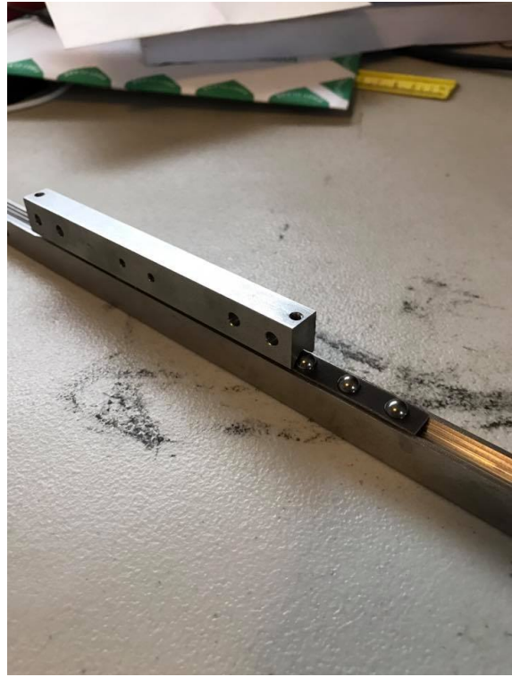
Figure 65: The V groove with the bearing balls and delrin bearing cage. This particular linear bearings are used for the sample stage.
