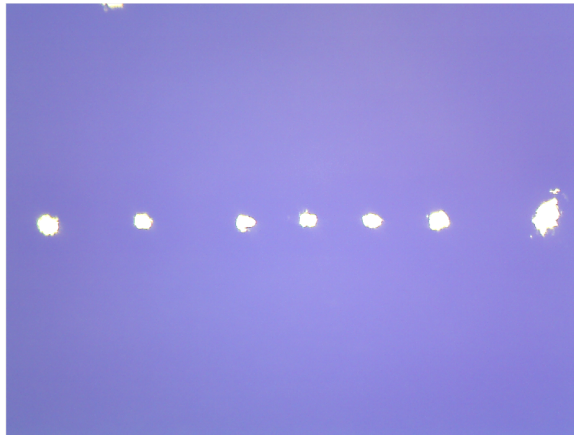
Figure 109: The cut holes varying in diameter as a function of Z position. The center hole with the smallest diameter represents the Z position most likely near the focal point of the objective lens.
