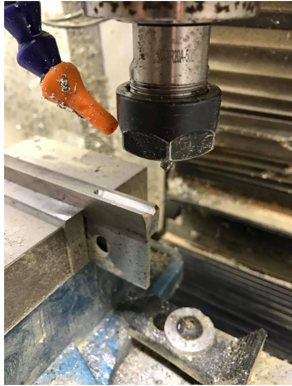
Figure 63: CNC machining the linear bearing V groove with a drill mill carbide endmill.
