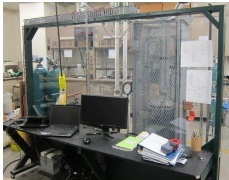
Figure 4.2. Polycarbonate panel to protect experimenters from equipment
