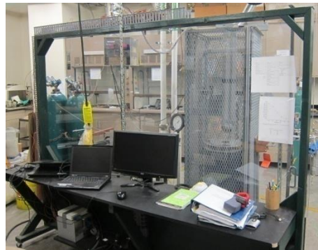
Figure 4.3. Secondary Lexan protective shield
