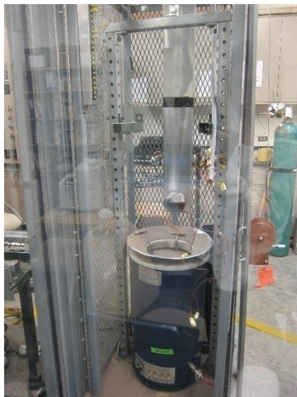
Figure 4.1. Welded steel-polycarbonate structure for enclosing WHTB during an experiment
