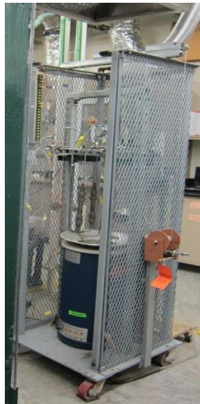
Figure 4.2. Sand bath equipment and protective structure
