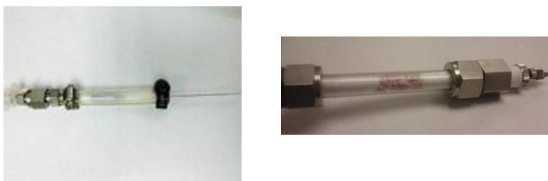
Figure 12.1. Gastight syringe with blue dry drierite desiccant (left) and with moist drierite desiccant (Right)
