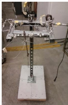
Figure 5.1. Custom-made WHTB -holder for reactor relocation.
