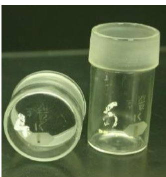
Figure 13.2 Glass Feed Moisture Content Container
