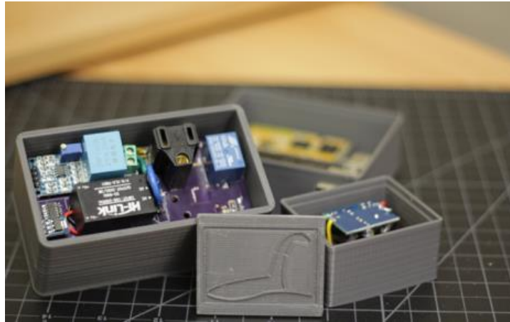
Figure B.3: SP(left), SEM (right), and sensor network gateway (back) designed for testbed integration
