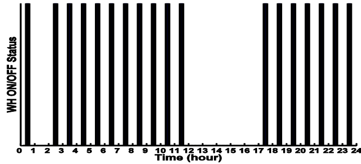
Figure 6.9: On/off status of WHS in aggregators A and B without demand scheduling
