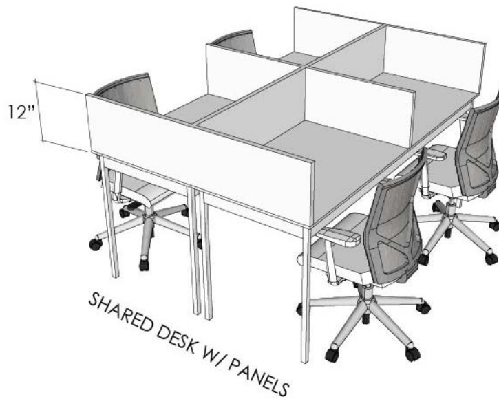
Figure 79: A 12" high panel above the desk is sufficient for productivity.
