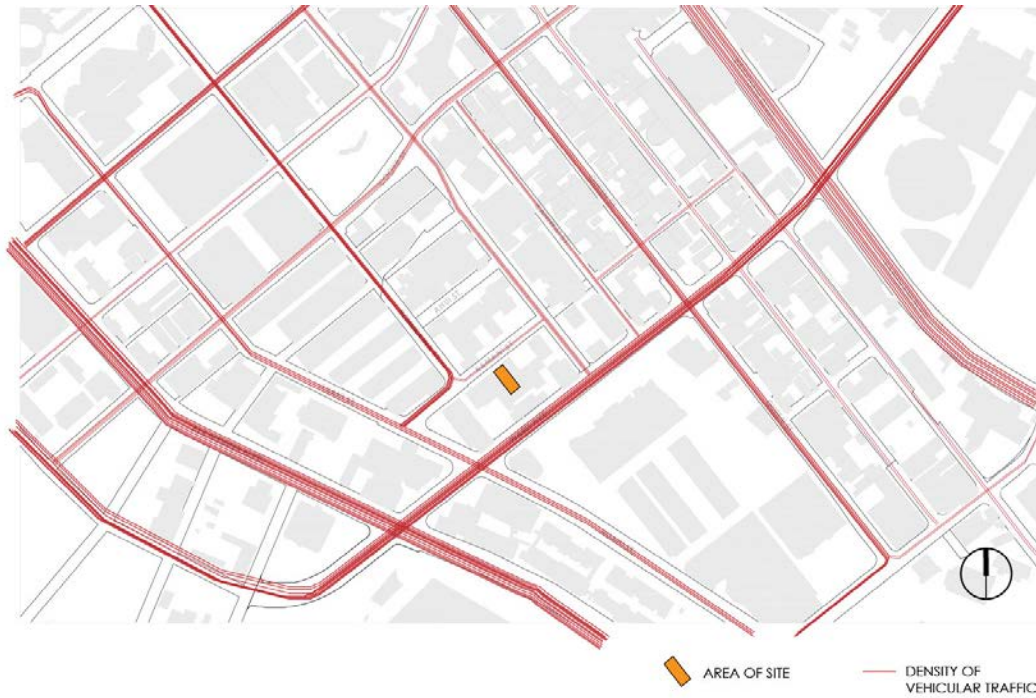
Figure 100: Vehicular traffic on Kamani St. is not highly active and often bypassed to and from Ward Avenue.
