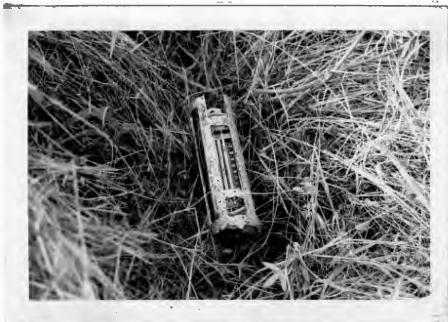
FIGURE 15. APPARATUS USED FOR MEASUREMENT OF TEMPERATURE AT THE GROUND SURFACE. METAL PROTECTIVE CASING SURROUNDING TAYLOR MAXIMUM - MINIMUM THERMOMETER.
