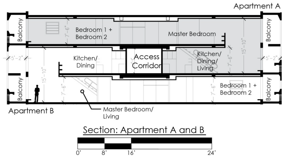
Figure 30. Le Corbusier’s Unité d’Habitation skip-stop double loaded corridor spatial configuration inspired by a “wine bottle rack”.
