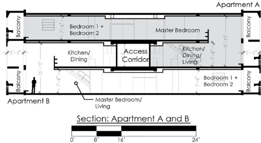
Figure 26. Sections of two common apartment units in the Unité d’Habitation building inspired by wine bottle racks.
