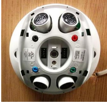
Fig. 6.9 Leviton OSC10-M0W multi-technology hybrid occupancy sensor
