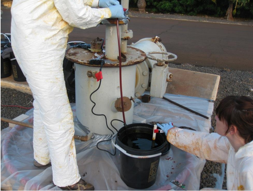
Figure 4-7: Transfer of the dye concentrate into injection Well 3.
