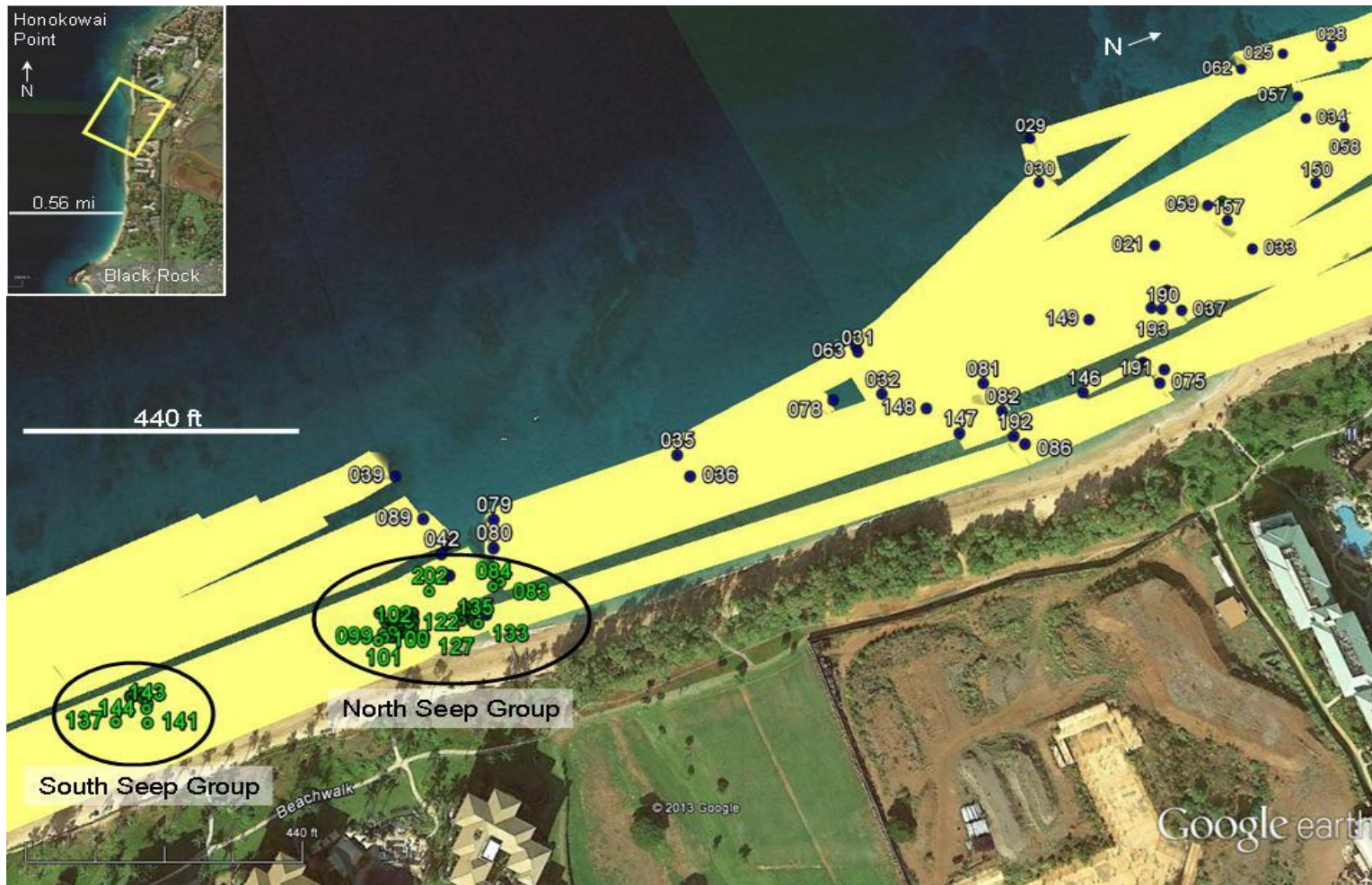
Figure 2-15: Area covered south of the Honua Kai and across Kahekili Reef during the submarine spring survey. The area surveyed is shown in the yellow box of the map insert. Blue dots with white numbers represent the start and end of the transects; the transect widths (in yellow) are directly proportional to the visibility of the scuba divers at the time of the survey. Green dots with numbers represent samples collected from submarine springs (Appendix Table A-6).
