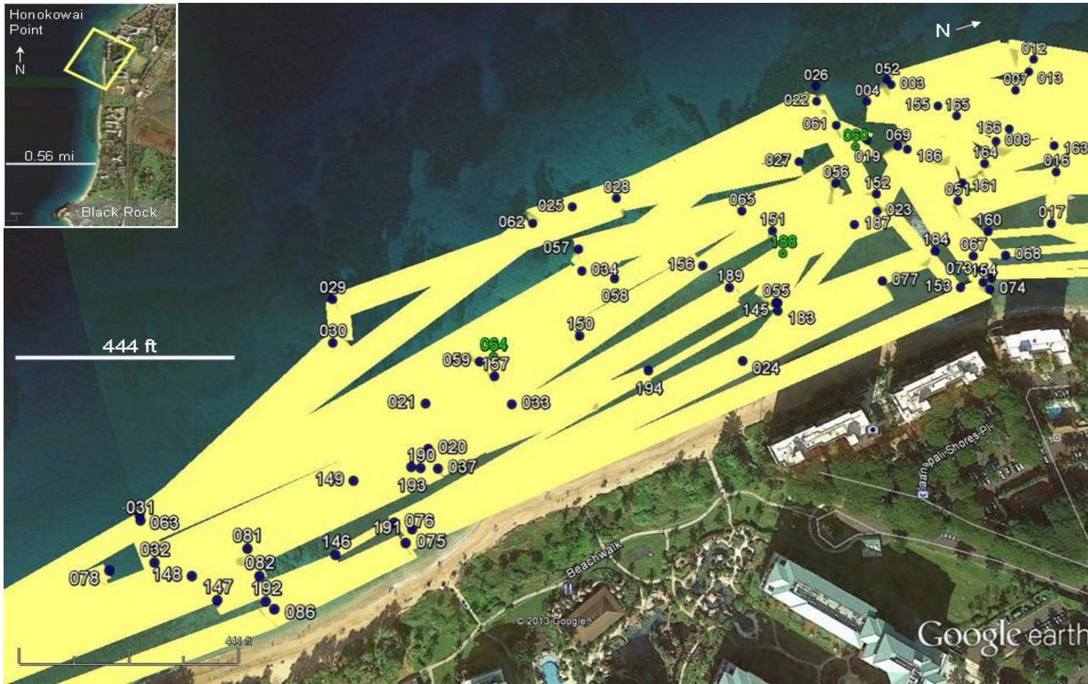
Figure 2-14: Area covered at adjacent to the Honua Kai during the submarine spring survey. The area surveyed is shown in the yellow box of the map insert. Blue dots with white numbers represent the start and end of the transects; the transect widths (in yellow) are directly proportional to the visibility of the scuba divers at the time of the survey. Green dots with numbers represent samples collected from shimmery water (Appendix Table A-6).
