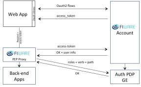
Figure 3: Platform level authorization (Level 2)[20]
