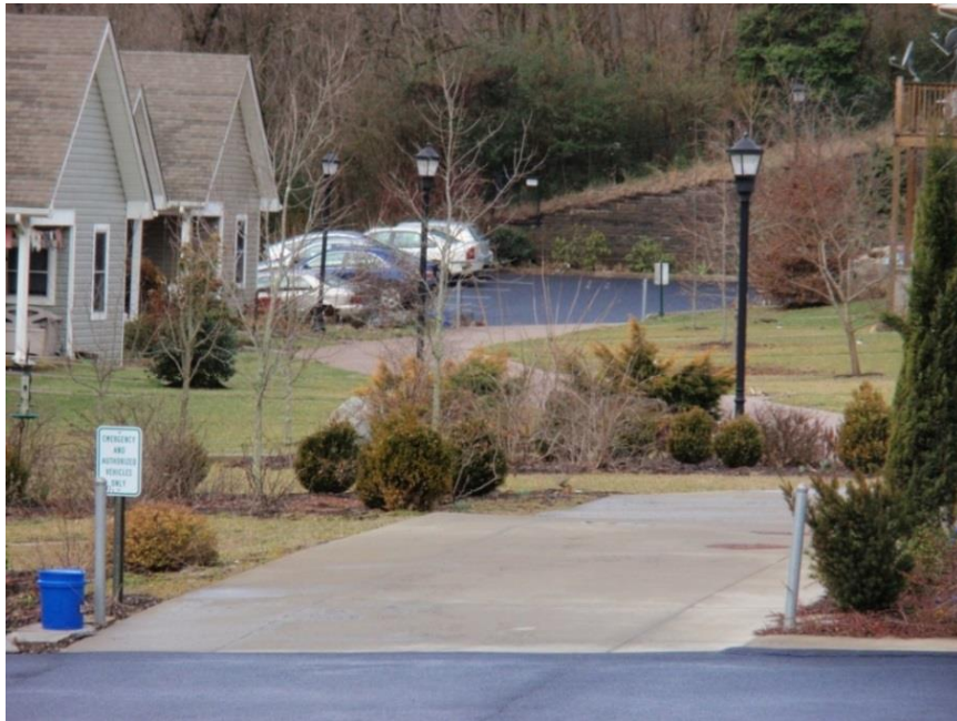
Figure 29: Signage of the pedestrian pathway. The width of the pedestrian path is wide to accommodate emergency vehicles and to allow for cars to drive closer to the dwelling units.
