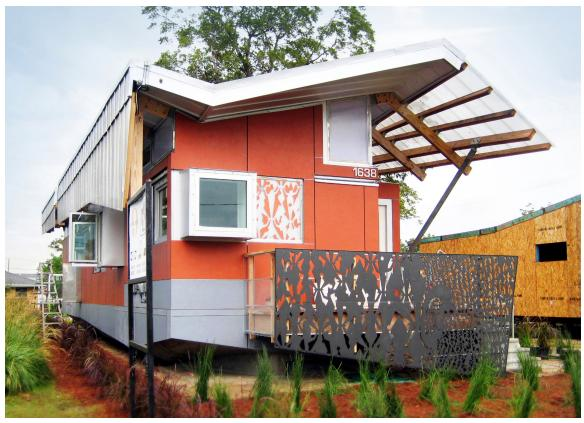
In New Orleans the FLOAT House can rise vertically on guide posts, floating up to twelve feet as water levels rise (Courtesy of Architectenbureau Marlies Rohmer)
