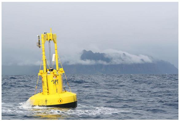
This Power buoy system is based on modular, ocean-going buoys that capture and convert wave energy into electricity. (Courtesy of U.S. Marine Corps and Cpl. Jody Lee.)
