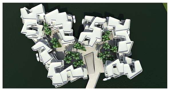
Caption: The Citadel, secured to the bottom with expandable tethers, will rise and fall with the changing water levels, making it impervious to flooding, tides, and sea level rise. (Courtesy of WaterStudio)
