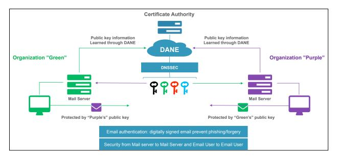
Figure 2: DANE system showing certificate retrieval for MTA and end-users (source: NIST [27])
