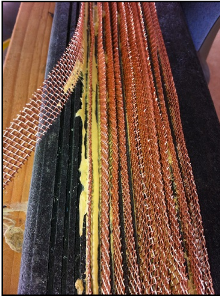
Figure 13. Partially completed cut mesh board, ten grooves filled with copper mesh with three not yet finished
