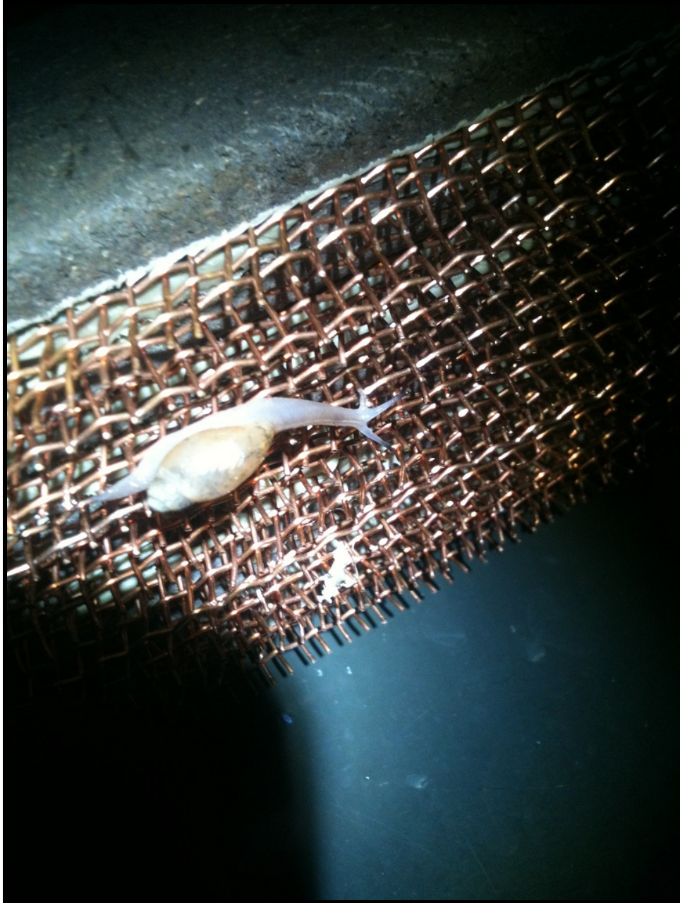
Figure 14. Small E. rosea attempting to cross the cut mesh barrier
