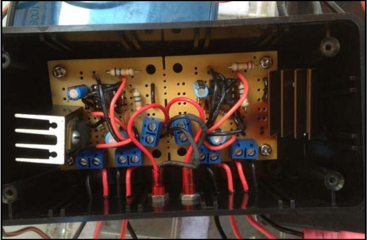
Figure 18. Chip (555) used in electric barrier
