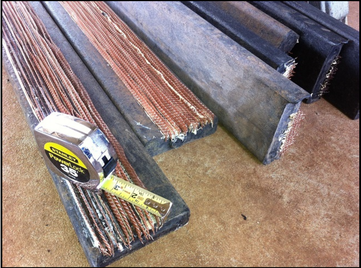
Figure 11. Finished cut mesh 2" x 6" plastic lumber boards ready to be transported to the field. The tan material in grooves is the construction adhesive.
