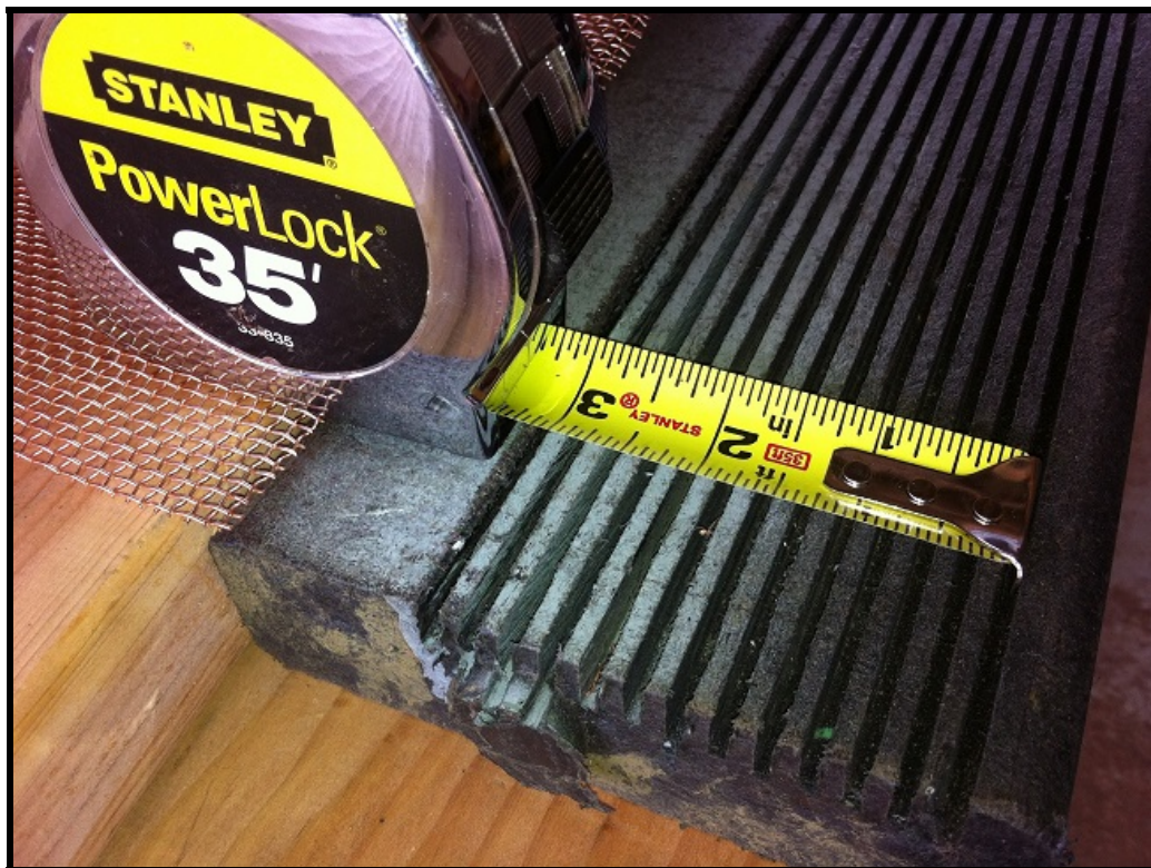
Figure 12. Raw materials for cut mesh barrier
