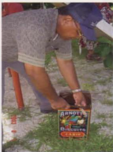
Step 2: Find an empty tin of biscuit and cut off the rims.
