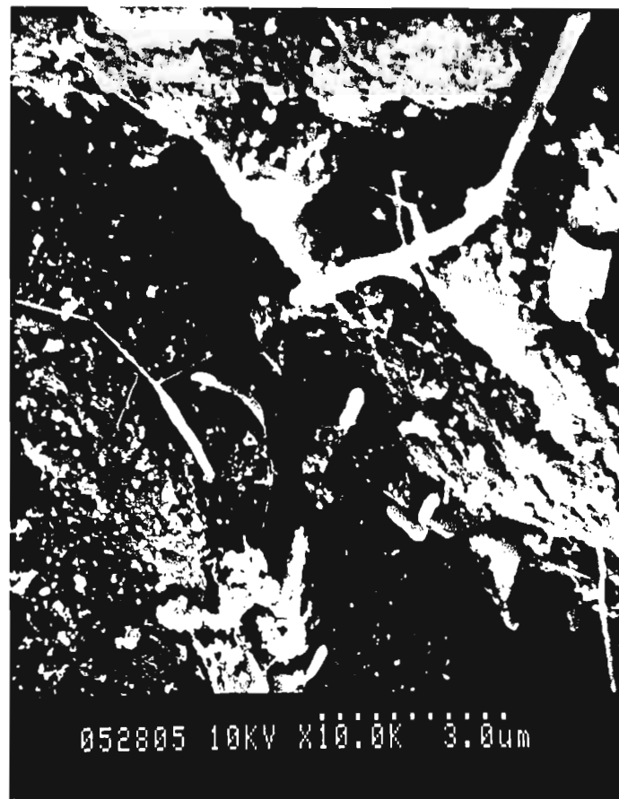
FIGURE 14. Rod-shaped bacteria and stalked forms on GAC from Kunia contactor no. 1 sampled in May 1991 (magnification 10,000x)
