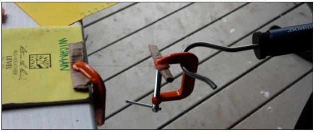
**Figure 3**. Experimental method for testing strength of **olonā** (*Touchardia latifolia* Gaudich.) cordage in Hā'ena, Kaua'i. Two C-clamps secure each end of the cord within a fold of cardboard. One end is secured to a fixed object (table) and the other to a scale used to measre the breaking strength.
