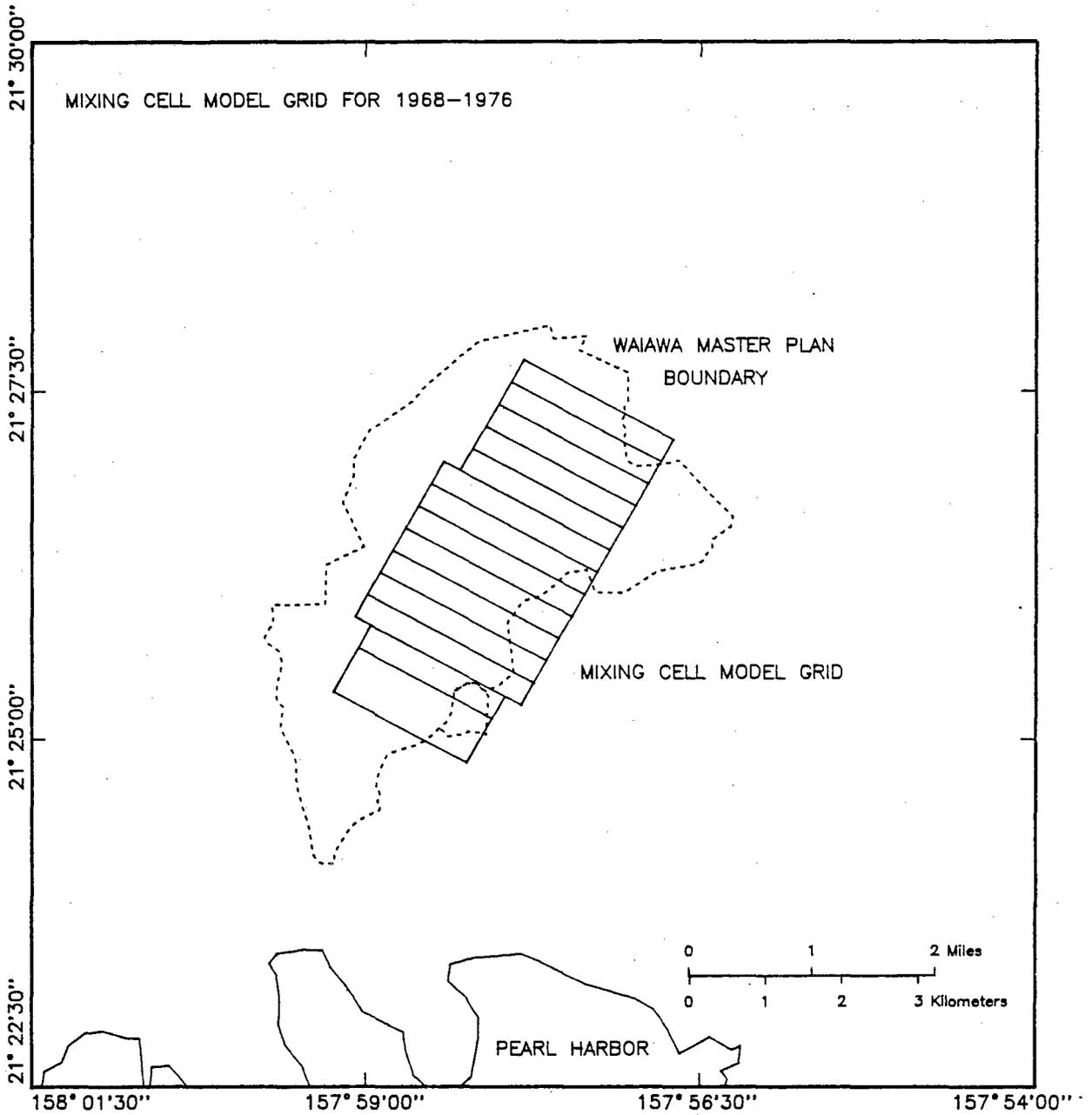
Appendix Figure E.22. Plan view of multiple mixing cell model grid for 1968-1976
