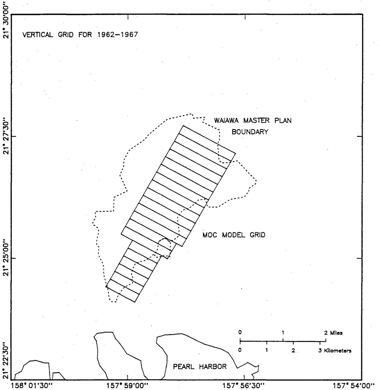
Appendix Figure E.13. Plan view of vertical MOC model grid for 1962-1967
