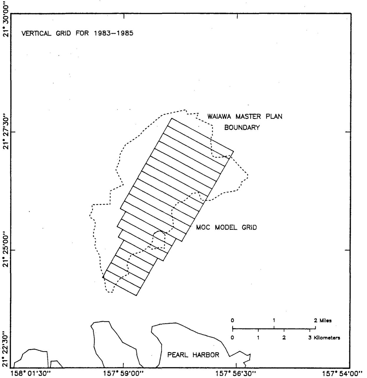
Appendix Figure E.16. Plan view of vertical MOC model grid for 1983-1985
