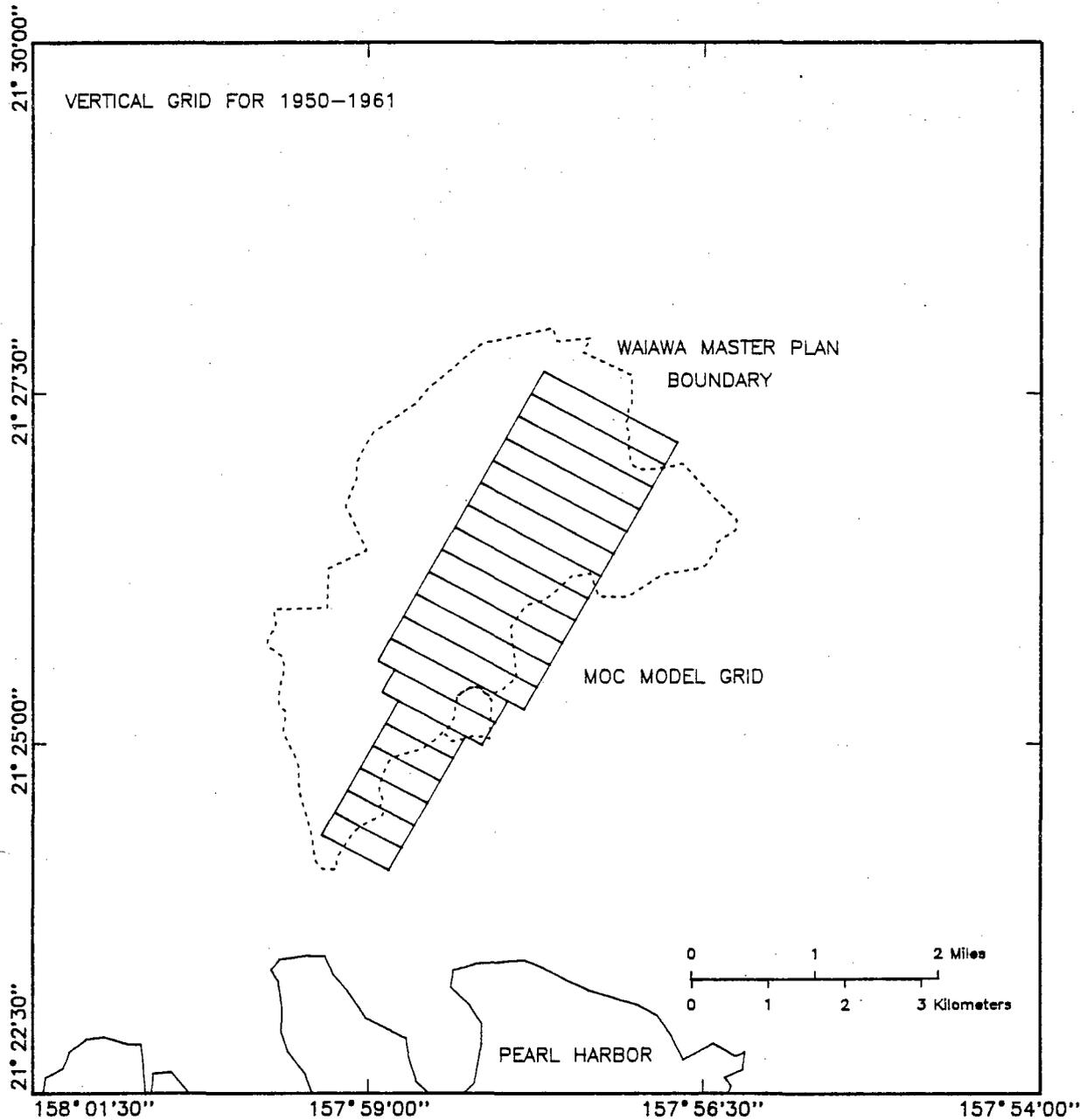
Appendix Figure E.12. Plan view of vertical MOC model grid for 1950-1961
