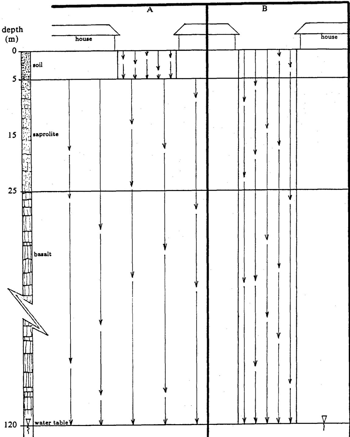
Figure 37. Cross section of water distribution methods: (A) distributed at top of saprolite; (B) advection dominated (distributed at water table)
