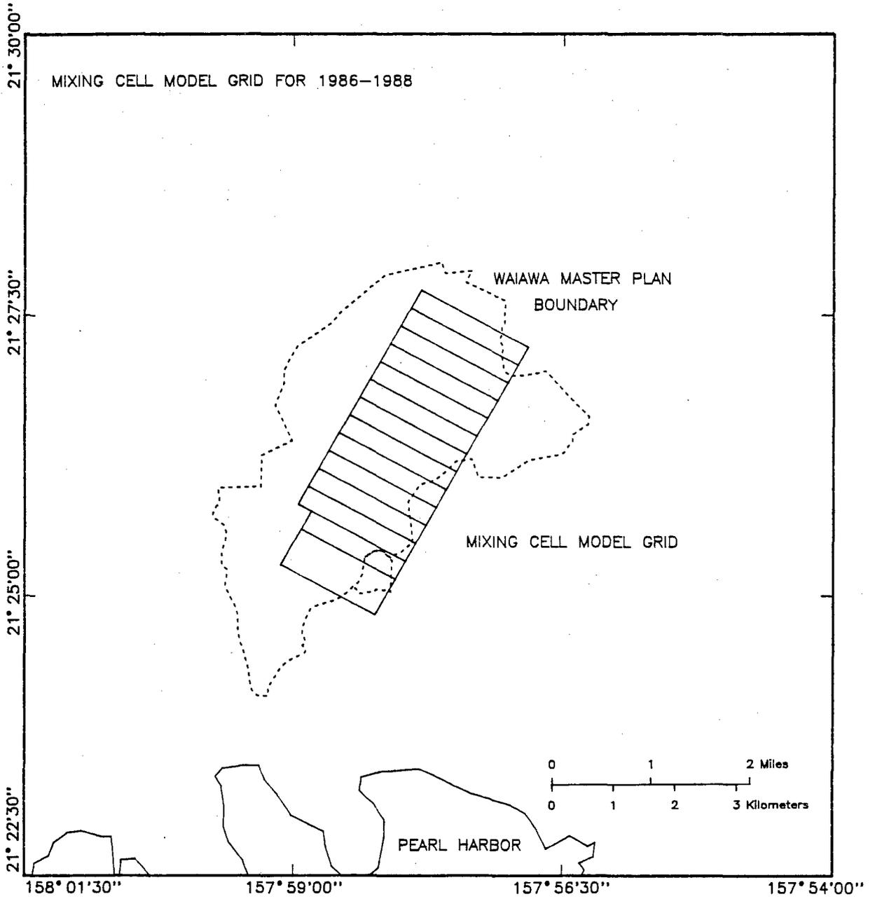
Appendix Figure E.25. Plan view of multiple mixing cell model grid for 1986-1988
