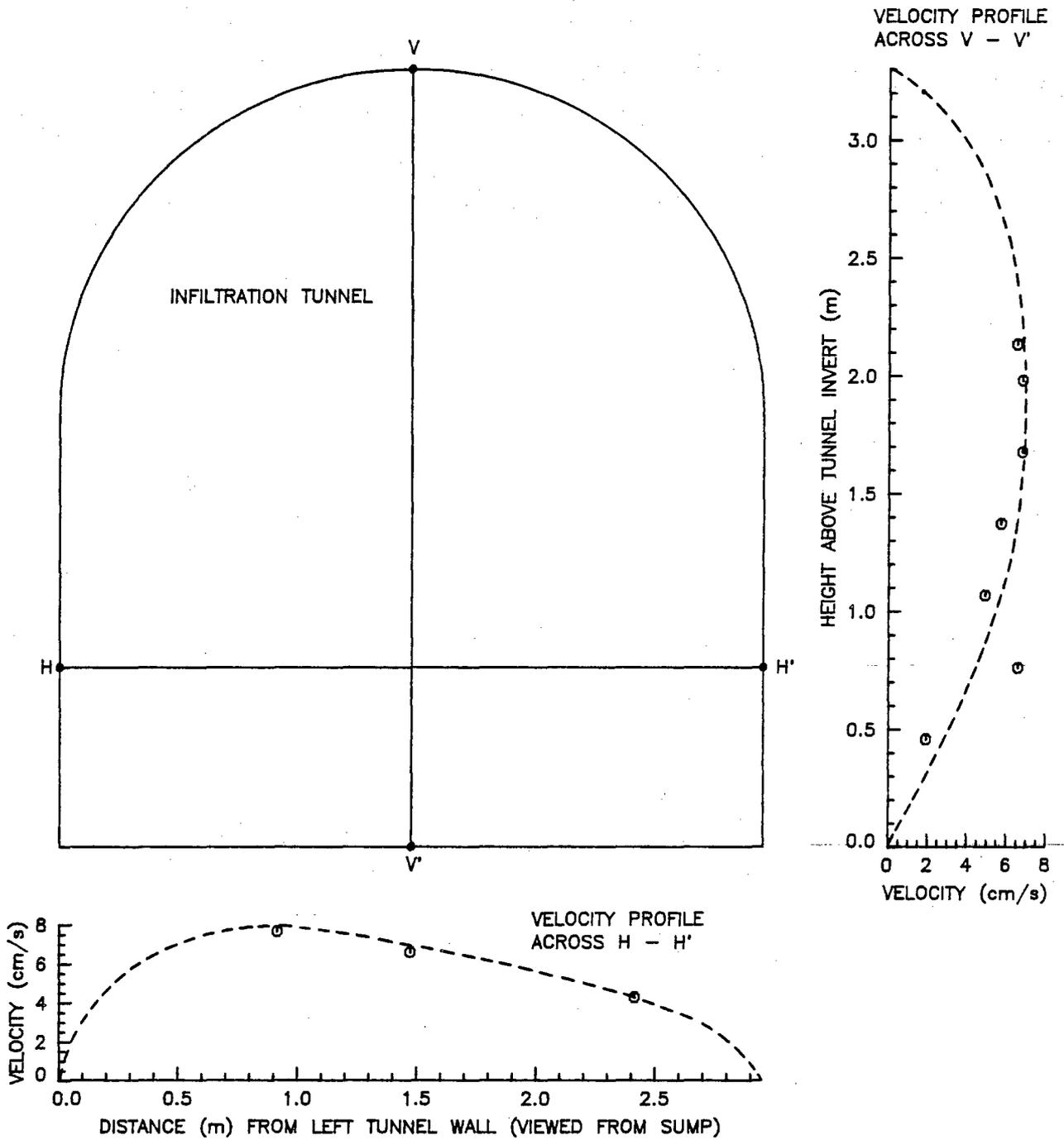
Appendix Figure F.1. Waiawa infiltration tunnel cross section and vertical and horizontal velocity profiles near sump
