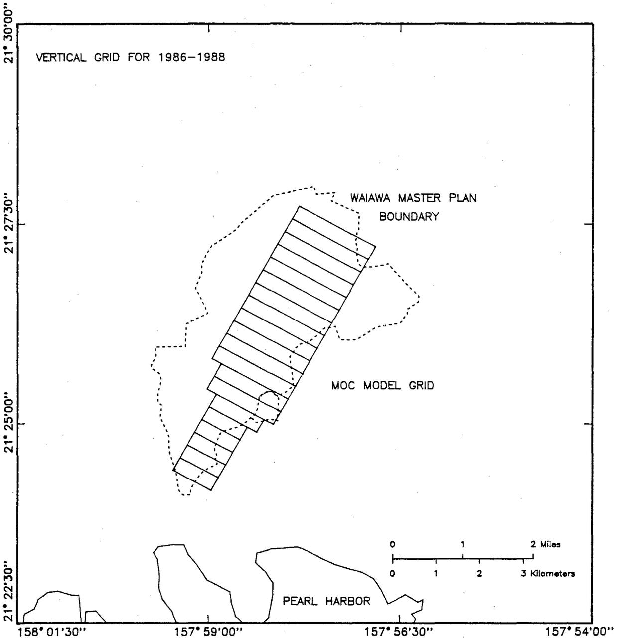
Appendix Figure E.17. Plan view of vertical MOC model grid for 1986-1988
