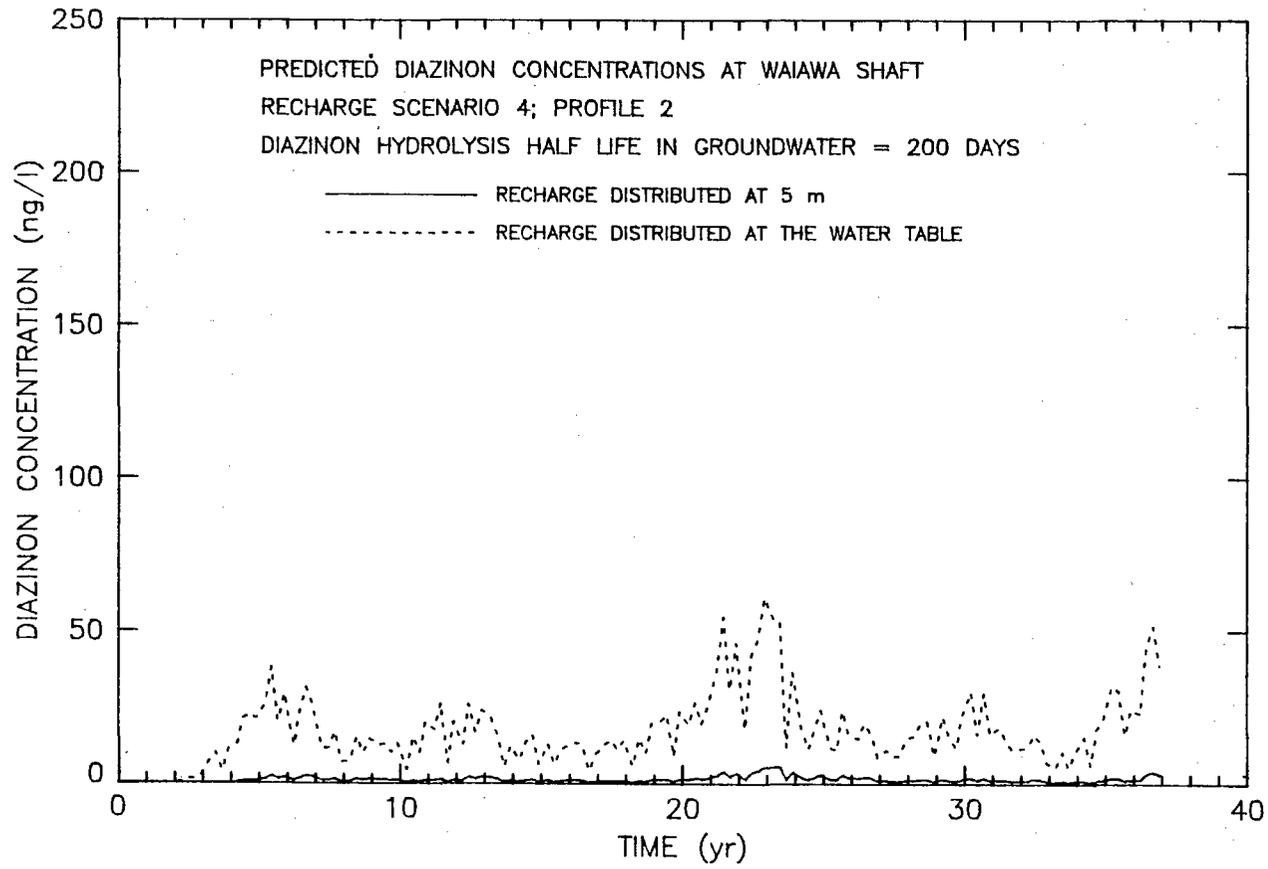
Figure 66. Diazinon simulations 11 and 14, Waiawa Shaft, Oahu, Hawaii
