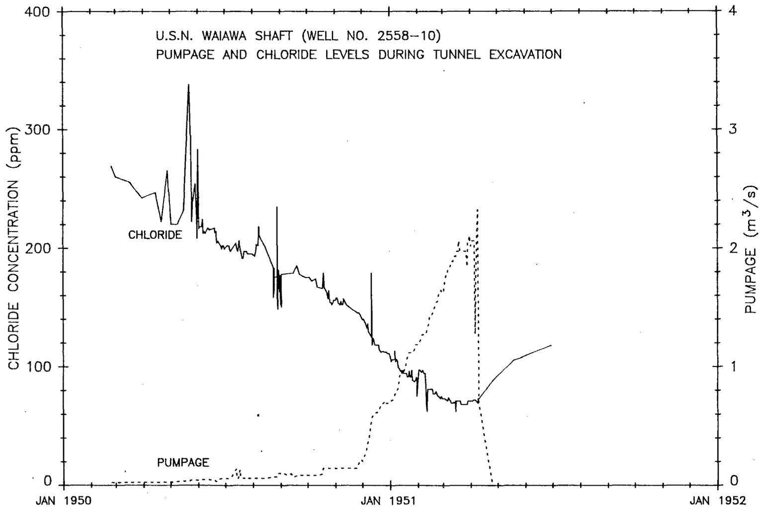
Figure 6. Pumpage and chloride concentrations at Waiawa Shaft during tunnel excavation
