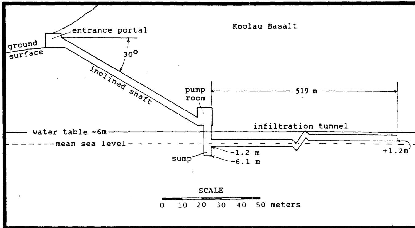
Figure 5. Diagram of U.S. Navy Waiawa Shaft and infiltration tunnel, Oahu, Hawaii
