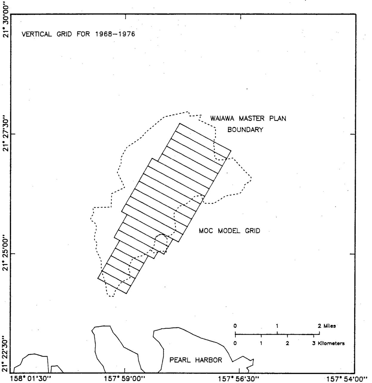
Appendix Figure E.14. Plan view of vertical MOC model grid for 1968-1976
