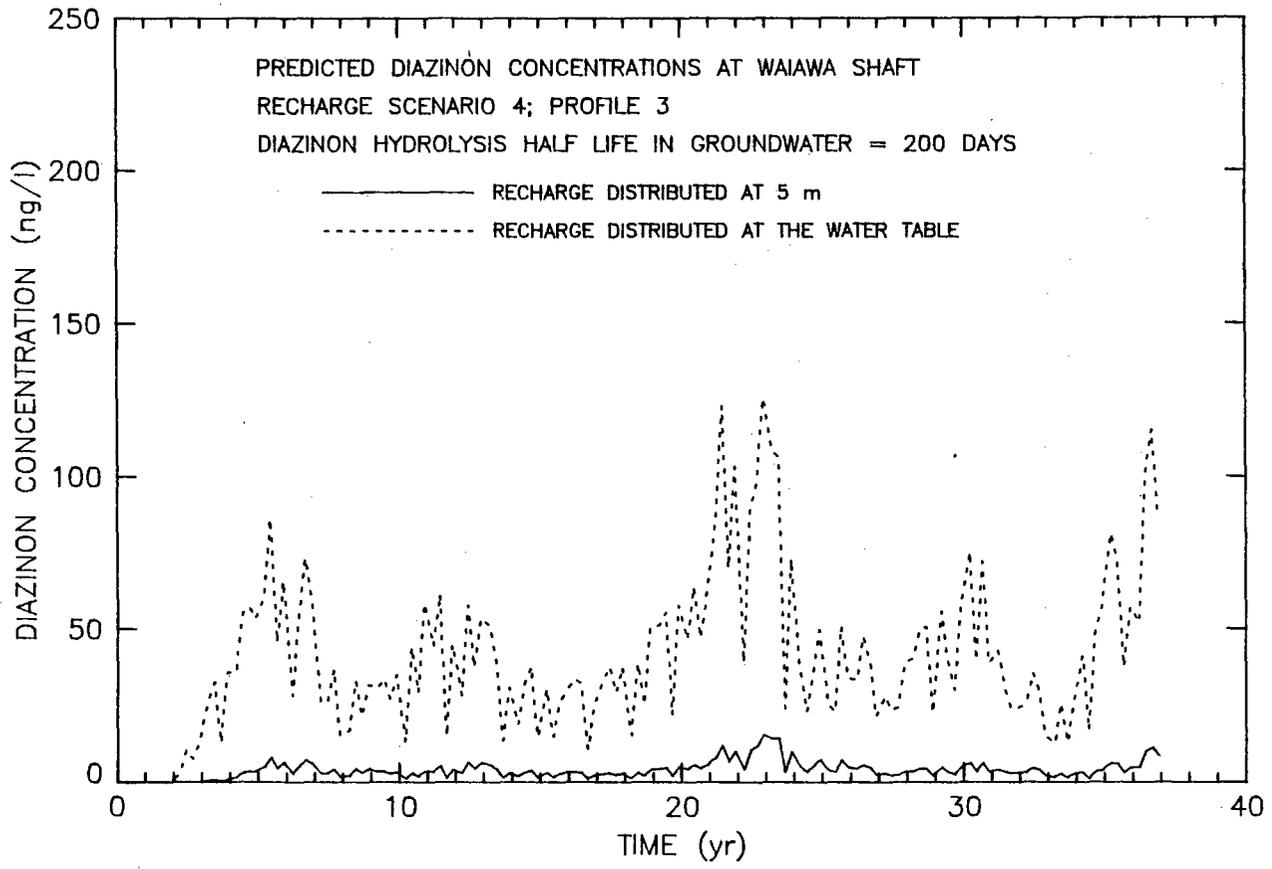
Figure 67. Diazinon simulations 12 and 15, Waiawa Shaft, Oahu, Hawaii
