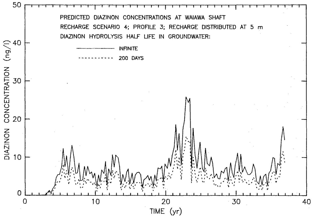
Figure 64. Diazinon simulations 15 and 20, Waiawa Shaft, Oahu, Hawaii
