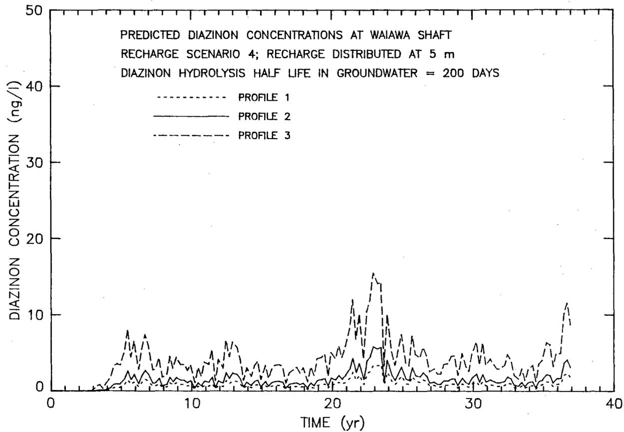
Figure 65. Diazinon simulations 13, 14, and 15, Waiawa Shaft, Oahu, Hawaii
