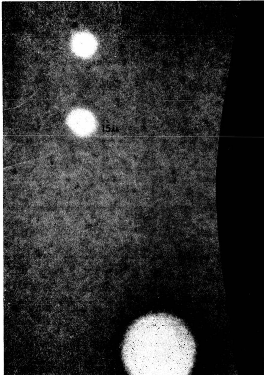
FIGURE 4. MICROPHOTOGRAPH OF FOG DROPLET IMPACT CRATERS ON MAGNESIUM OXIDE COATED SLIDE. TYPICAL FOG DROPLETS SHOWN IN RELATIONSHIP TO 1 mm, RAIN DROP (CHORD AT RIGHT)
