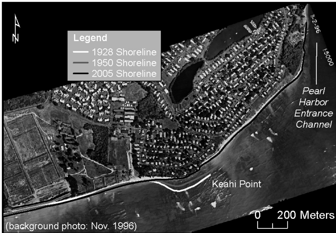
Figure 4.9. Aerial photograph (1996) and historical shoreline positions (1928, 1950, and 2005) documenting erosion along a beach cusp at Keahi Point, south Oahu, Hawaii (see Figure 4.1 for location).
