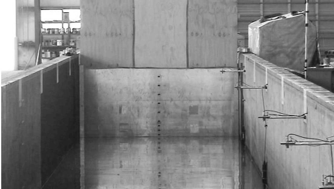
Figure 3.2. View of instrumented aluminum wall and plywood extension to prevent overtopping
