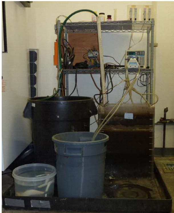
Figure 2.6 Lab bench MBR setup
