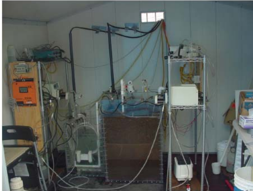
Figure 2.5 Bench Enviroquip (right) and Ionics (left) MBRs at Honouliuli WWTP
