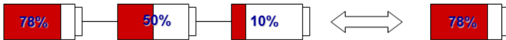
Figure 24 Method #5: 3-cell pack SOC is single cell's greatest SOC within the string
