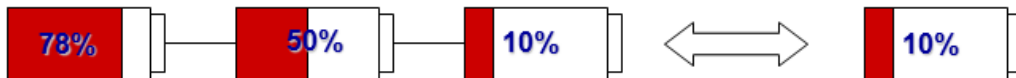
Figure 23 Method #4: 3-cell pack SOC is single cell's lowest SOC within the string
