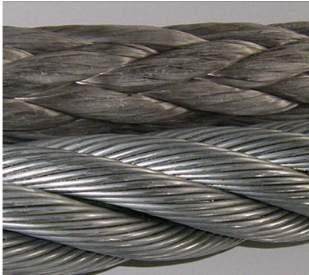
Figure 3.3. A side-by-side comparison of Dyneema synthetic rope (28mm diameter) with steel wire rope (36mm diameter) [52].
