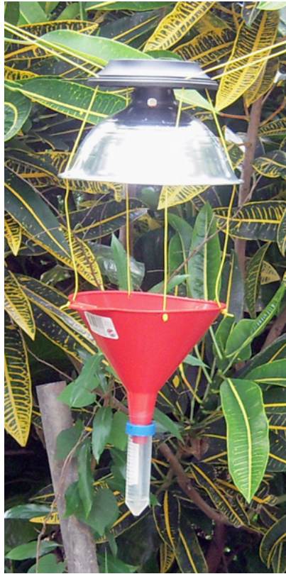
Figure 4. Light-trap. From top: solar light source, hood, funnel and removable centrifuge tube.
