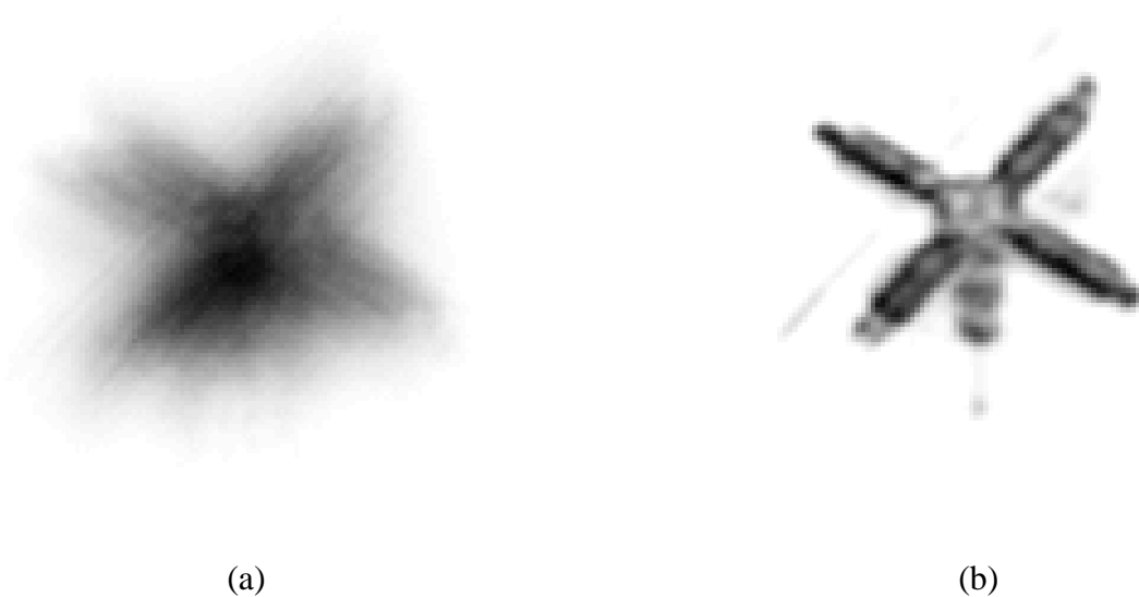
Figure 2: (a) typical raw frame and (b) 16-frame MFBD reconstruction, D/r_0=16 , SNR=40 dB
