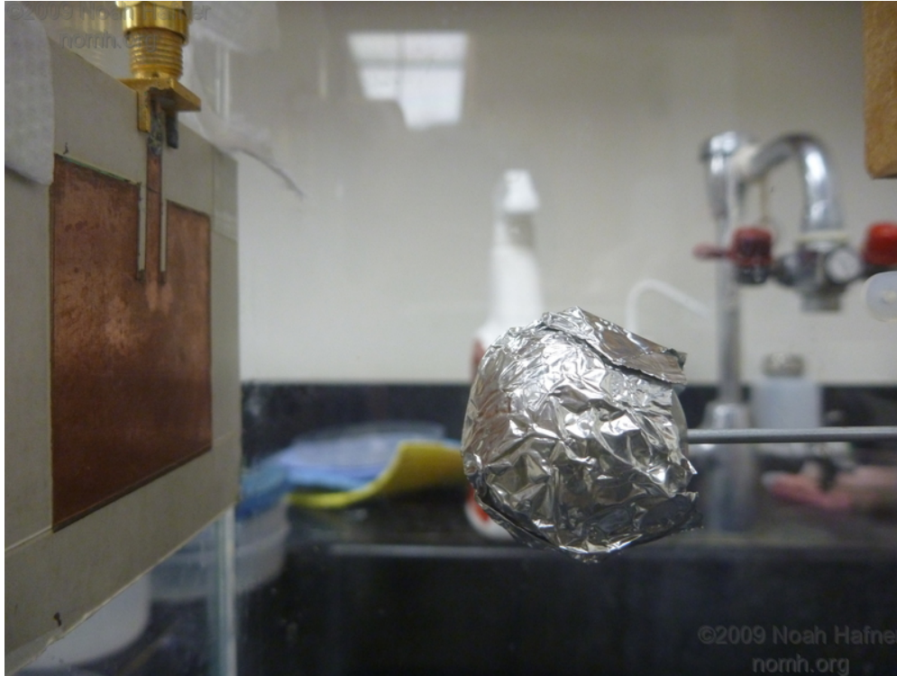
Figure 2.9: Moving reflector for underwater characterization of Doppler radar system for fish sensing.
