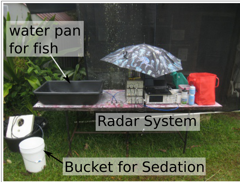
Figure 3.1: Photo of fish testing table. A white foam plate, visible near the Bucket for Sedation, found use as a sunshade for the fish during testing. The umbrella was required for maintaining a bit of readability in the computer display as well as the SR560 amplifier indicators.
