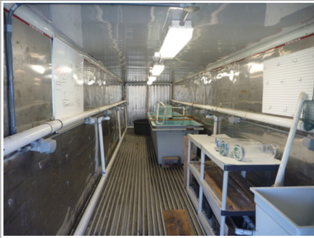
Figure 4.14: Interior view of converted shipping container used as testing area for the experiments. This area was located near the tanks used for raising the fish and provided a controlled environment for initial experiments.
