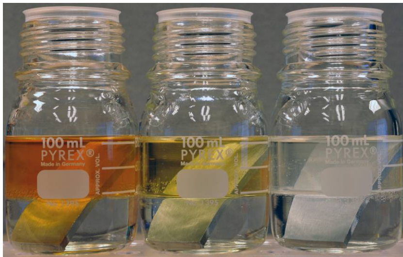
Figure 1. Experimental setup of fuel-water mixtures with 1018 steel coupons immersed. Left to right: B100/water mixture, B20/water mixture, and ULSD/water mixture.
