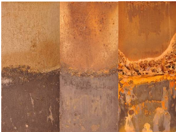
Figure 15. 6 month steel coupon samples exposed in an anaerobic environment segregated by type of fuel.
