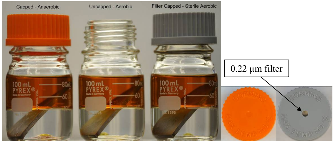
Figure 2. B100/water fuel mixture depicting anaerobic, aerobic, and selective aerobic environments. Anaerobic cap and selective aerobic cap depicted.
