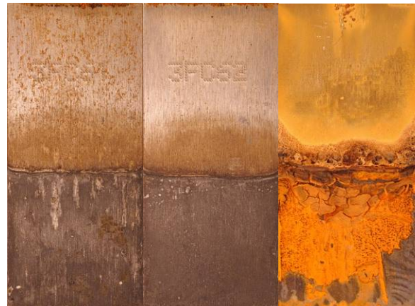
Figure 15. 6 month steel coupon samples exposed in an anaerobic environment segregated by type of fuel.
