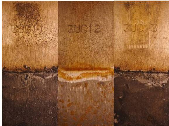
Figure 18. 1 year steel coupon samples exposed in an anaerobic environment segregated by type of fuel.
