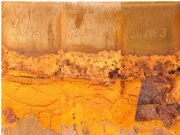
Figure 17. 6 month steel coupon samples exposed in a selective aerobic environment segregated by type of fuel.
