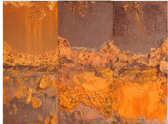
Figure 18. 1 year steel coupon samples exposed in an anaerobic environment segregated by type of fuel.
