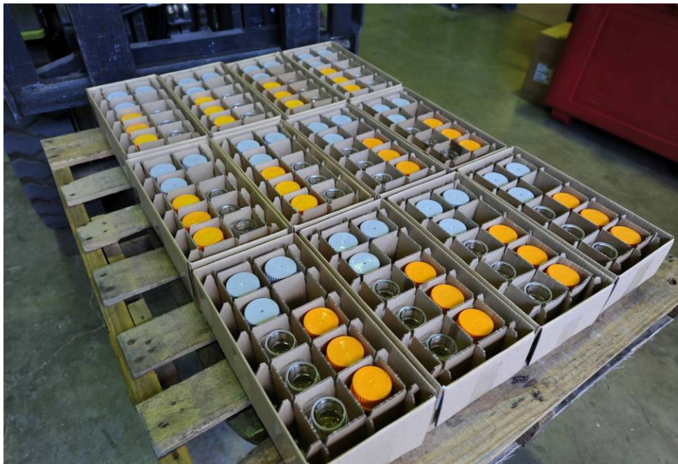
Figure 3. 108 samples loaded in boxes to be exposed outdoors for six months and one year.
