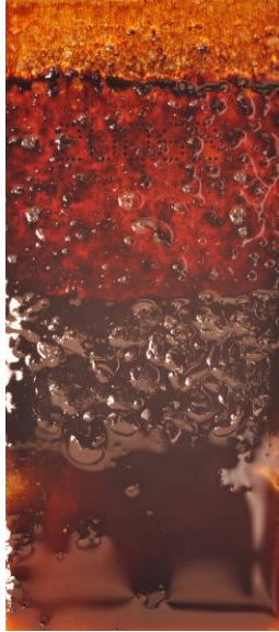
Figure 21. Microbial contamination in the form of sludge on 1018 steel coupon exposed in filtered/unfiltered B20 fuel-water mixture in aerobic environment.
