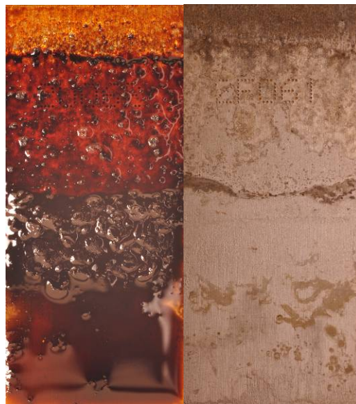
Figure 77. Before and after acetone wash image of 1018 steel coupon exposed in B20 fuel-water mixture exposed in an aerobic environment.
