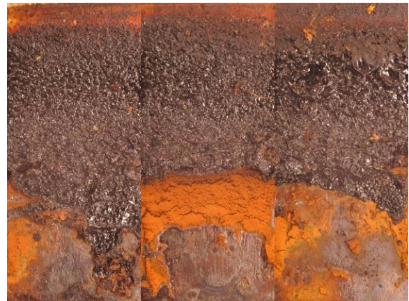
Figure 19. 1 year steel coupon samples exposed in an aerobic environment segregated by type of fuel.
