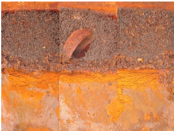
Figure 16. 6 month steel coupon samples exposed in an aerobic environment segregated by type of fuel.
