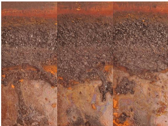
Figure 19. 1 year steel coupon samples exposed in an aerobic environment segregated by type of fuel.
