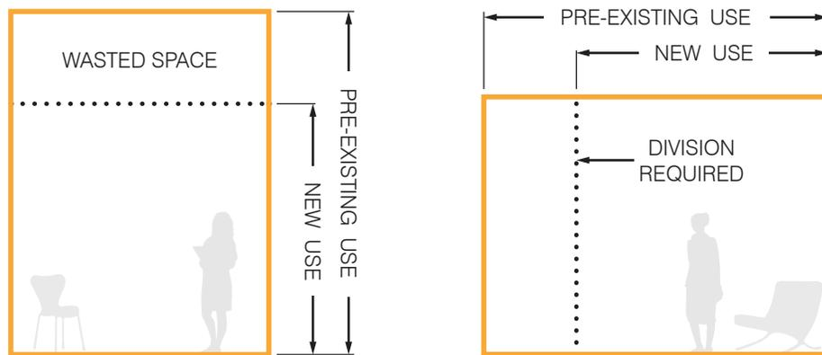
FIGURE 51 CHANGING LARGE SCALE OF SPACE (ROOM SECTION)
