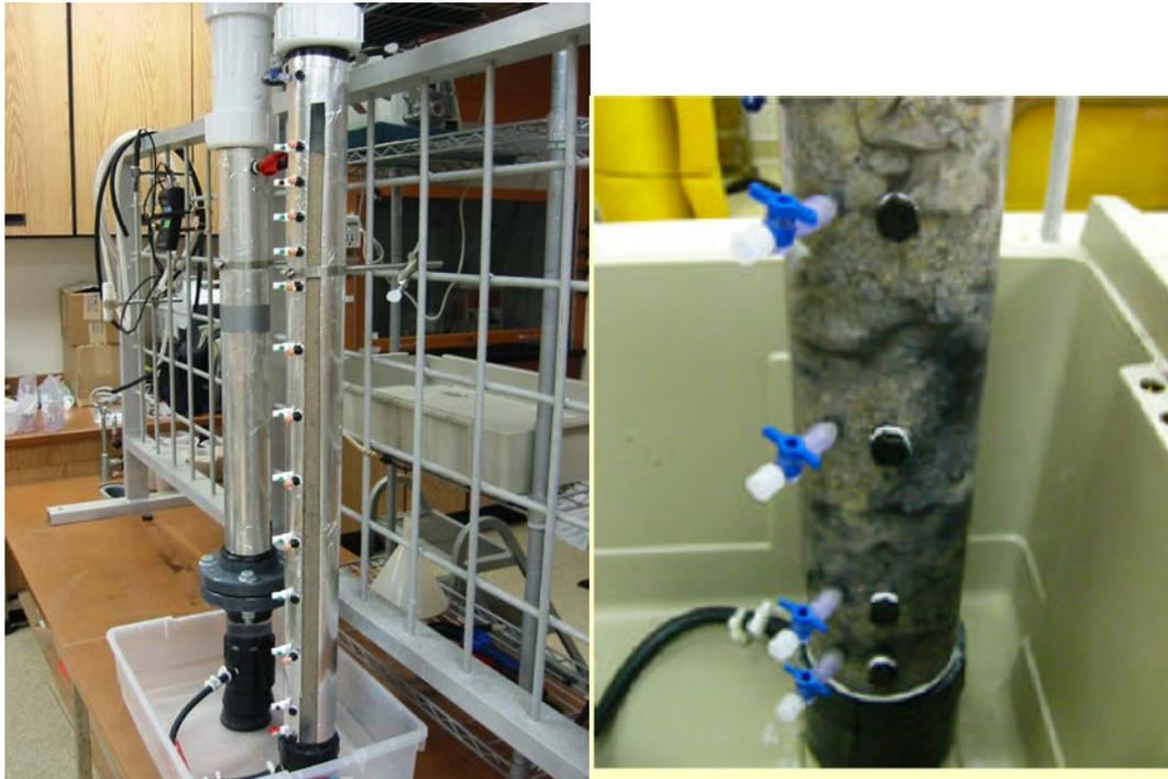
Figure 3.2. Microcosm set up (right) and close up view of porewater sampling ports (left) (courtesy A. Hannides).
