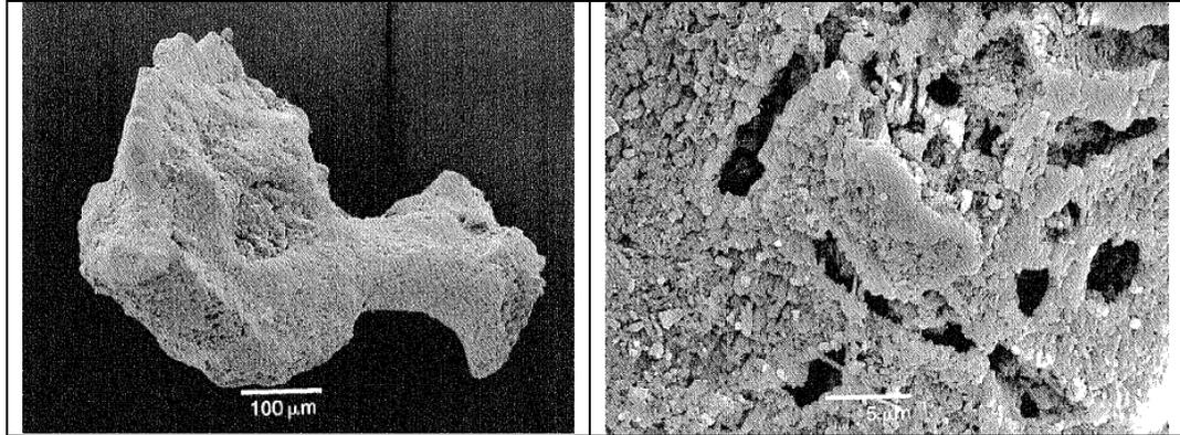
Figure 1.1. Carbonate sand grain exhibiting skeletal features (left). Close up view of the channels and crevices that characterize carbonate sands and thus provide a high external and internal surface area (right) (Wild et al, 2006).
