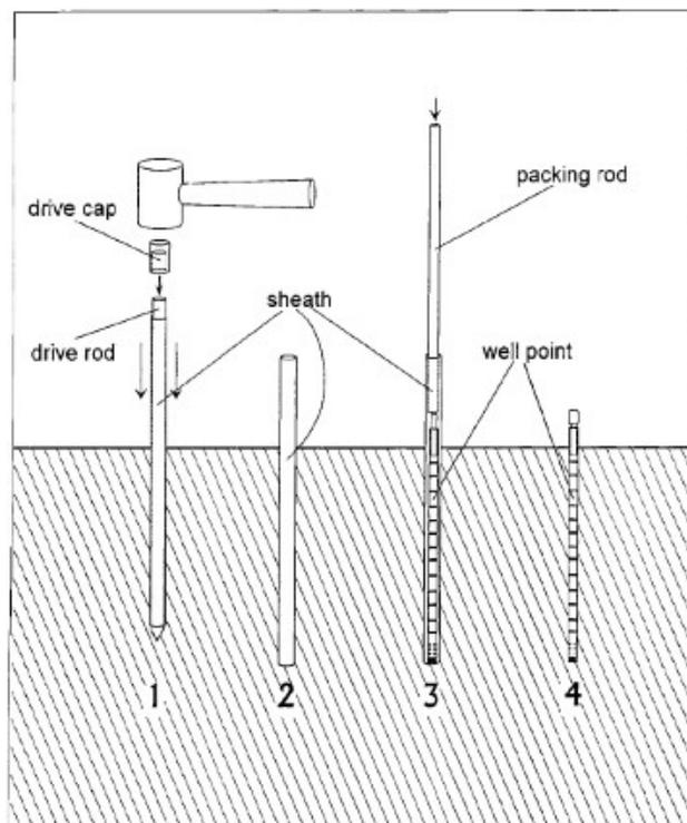
Figure 3.3. Diagram of well point sampling (Falter and Sansone, 2000b).
