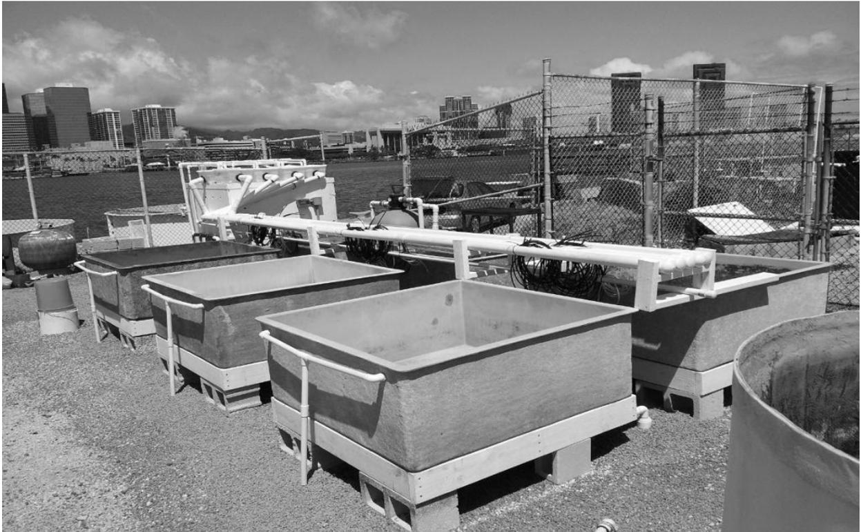
Appendix 3.S1 Outdoor seawater system at the Ānuenuue Fisheries Research Center, Sand Island, O'ahu that consists of six water baths.
