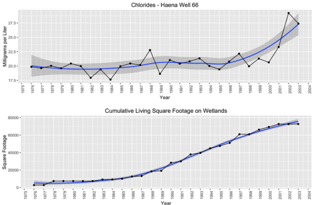
**Figure 44.** Well Chlorides versus Cumulative On-site Disposal Systems
