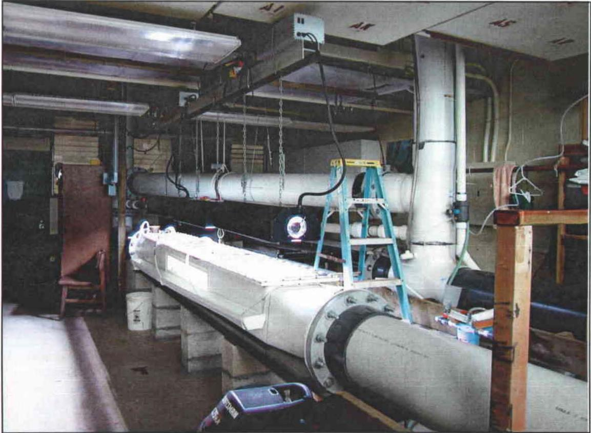
Figure 1. Wave-flume at HIMB. Flume was constructed in Summer 2002 and is capable of producing steady and oscillatory flow. The 18-m flow path flume can contain a volume of  $1.5 \text{ m}^3$  and has a test section area of  $0.9 \text{ m}^2$ . Metal halide bulbs provide lighting to the indoor system.
