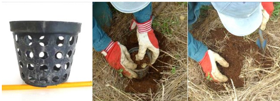
Figure 1. Bait and trap device : how to use it? Black PVC "trapping" pots (250 ml volume, 9 cm high x 11 cm wide) with 76 holes 1.3 cm in diameter, 16 of which were at the bottom were buried 15 cm in the soil (entire pot was covered with soil). Prior to burial, the pots were gently filled to a depth of 3 cm with soil removed from hole in which the pot was to be buried. Bait consisting of three potato slices 2.5 cm in diameter and 2.5 cm thick was placed on the soil, the pot was filled to the top with additional soil and then buried.
