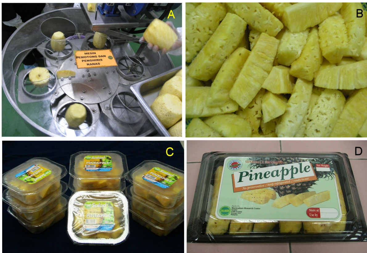
Figure 1A, machine for cutting pineapple spears; 1B, fresh cut spears ready for packing; 1C and 1D, polypropylene containers packed with fresh-cut pineapple.
