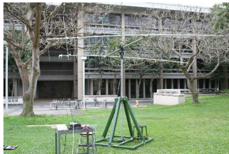
Figure 5: Complete raised VHF/UHF mobile-modular ground station
