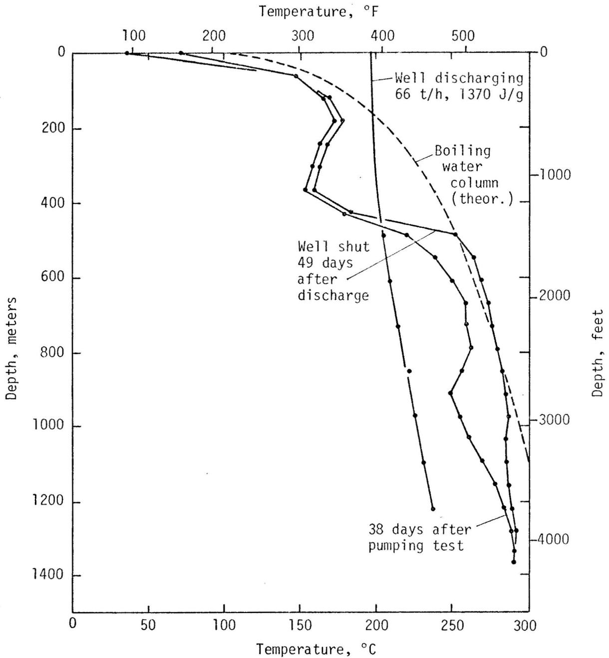
Figure 18. Downhole Temperatures at Various Well Conditions
