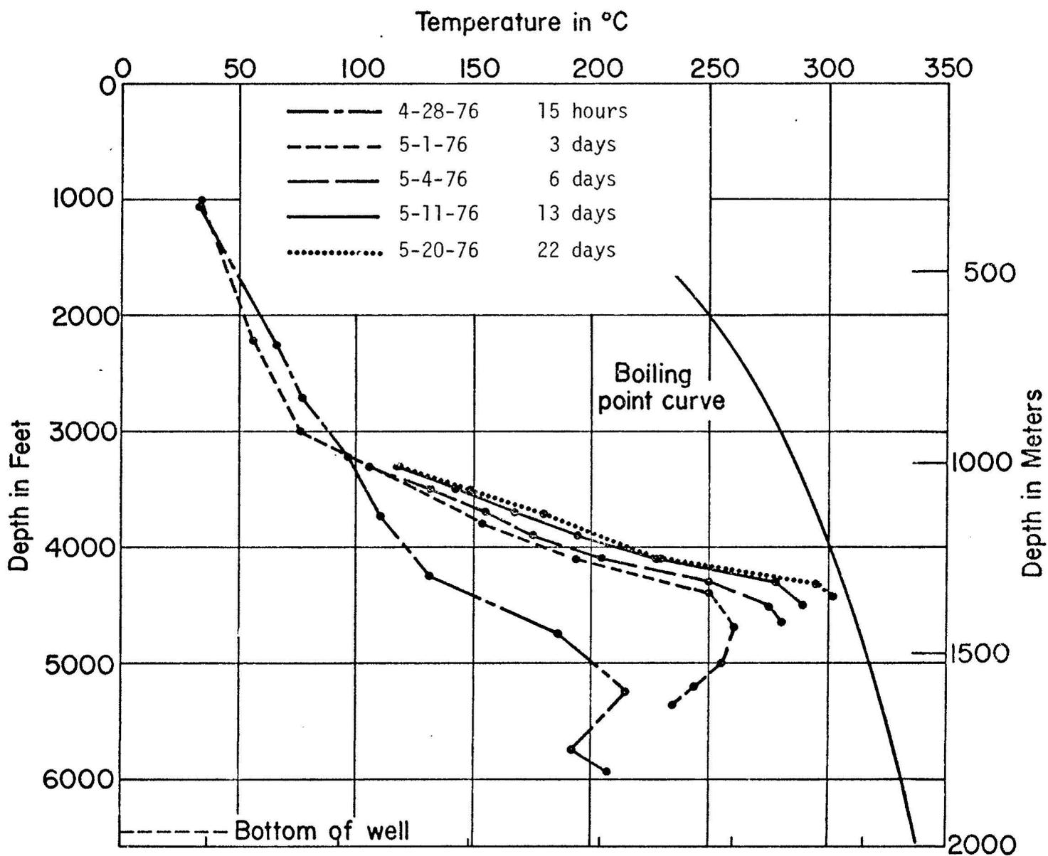
Figure 9. Temperature-Depth Plot for HGP-A (after liner installed)
