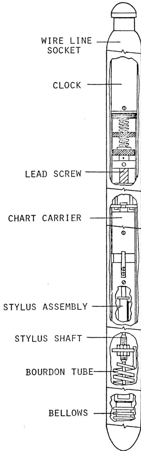
Figure 7. Kuster Pressure Recorder
