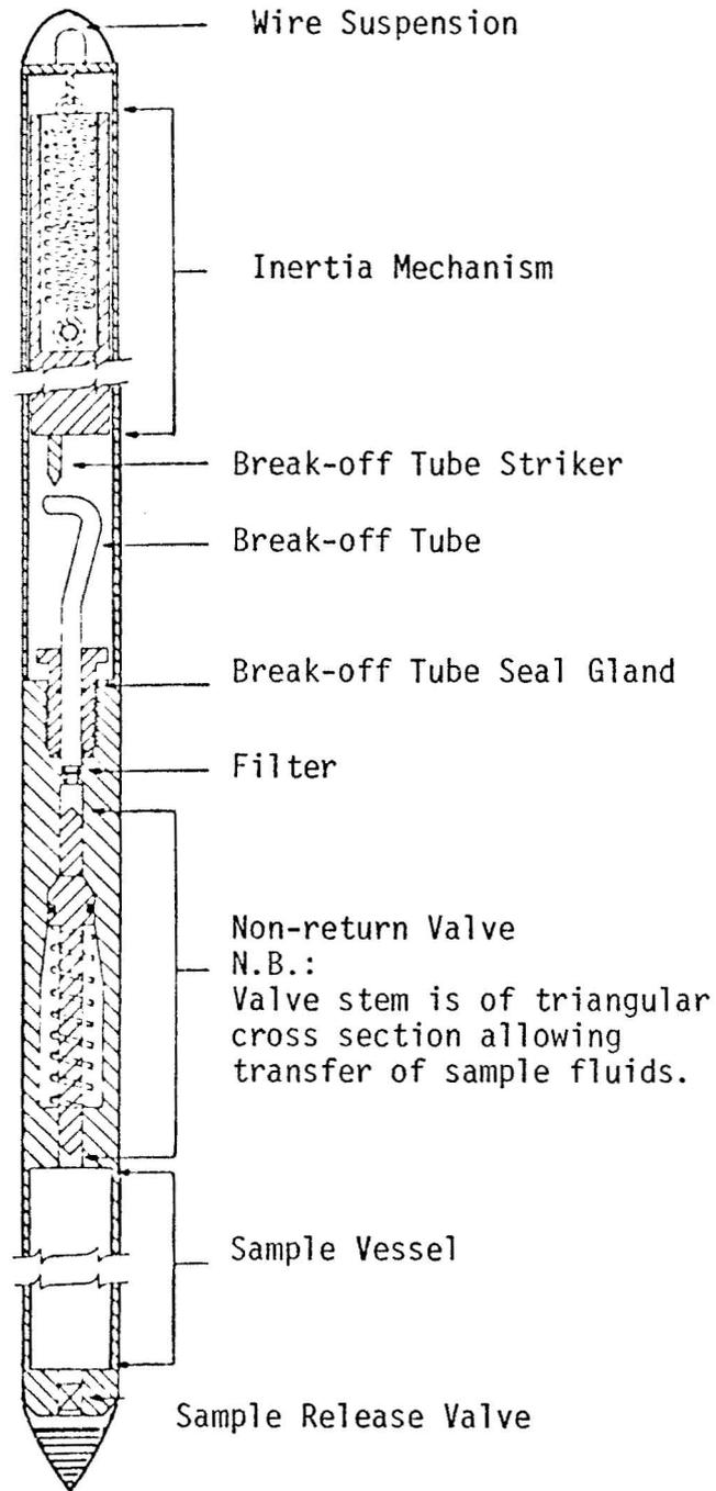
Figure 15. Klyen Deep Well Subsurface Sampler
