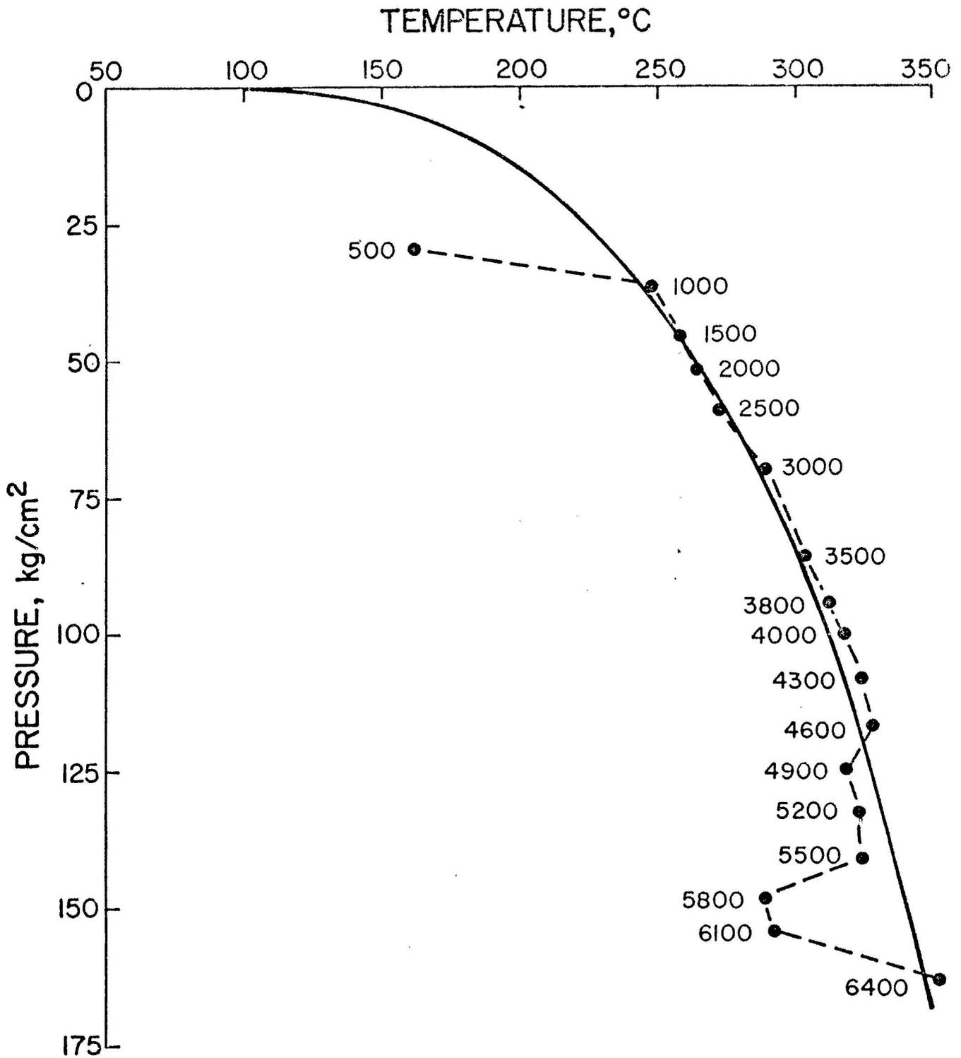
Figure 13. Temperature vs Pressure for HGP-A, July 22, 1976
