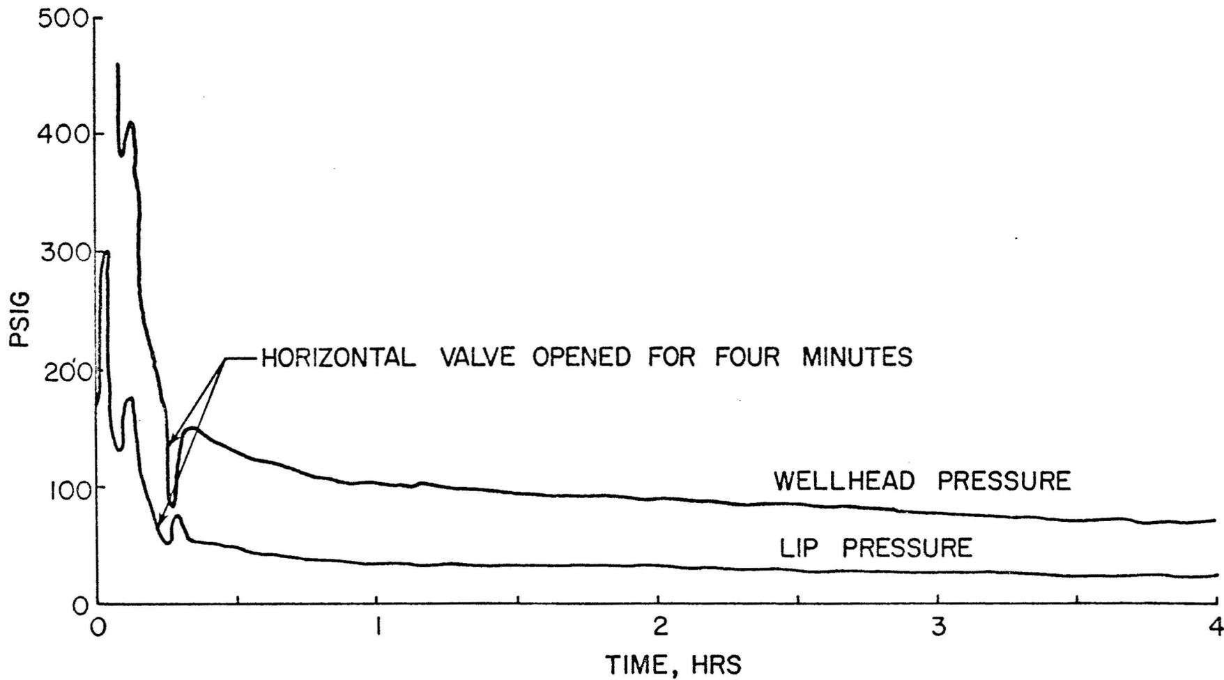
Figure 12. HGP-A Flow Test, July 22, 1976
