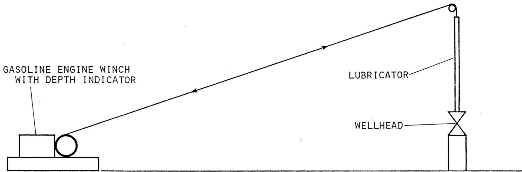
Figure 8. Kuster Measurement Equipment
