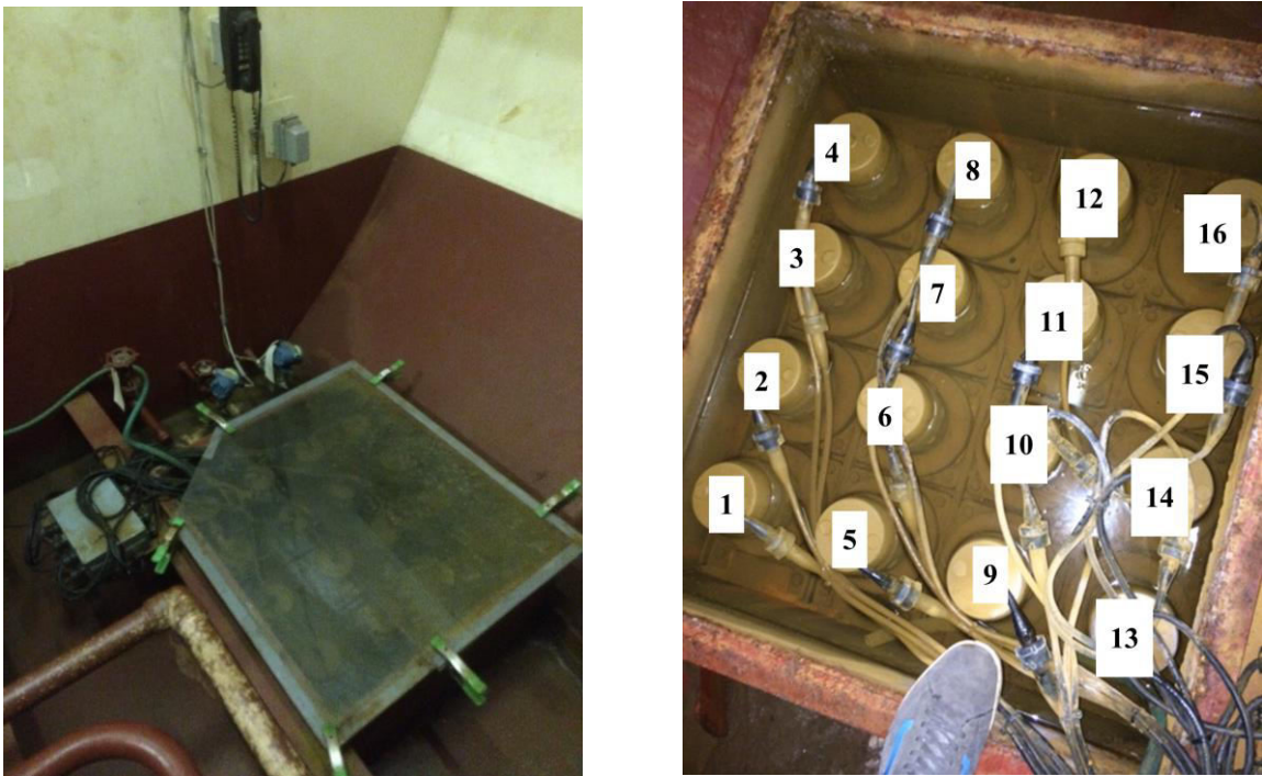
Figure 5. Housing and interior view of the 4x4 transducer array located on the hull of the R/V Kilo Moana . The coffer dam keeps the transducers under water to reduce risk of cavitation and to improve the coupling to the ship's steel hull.
