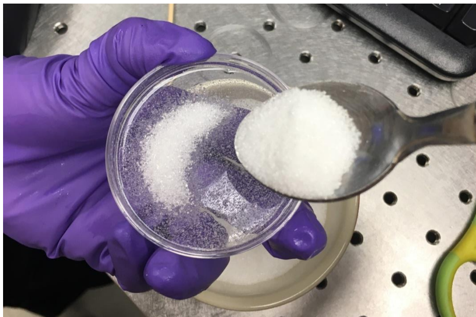
Figure 2.5: The addition of white granulated sugar to the uncured PDMS was done until the solution was completely filled with sugar. After curing the PDMS dielectric, the sugar crystals were dissolved to reveal the micropores.
