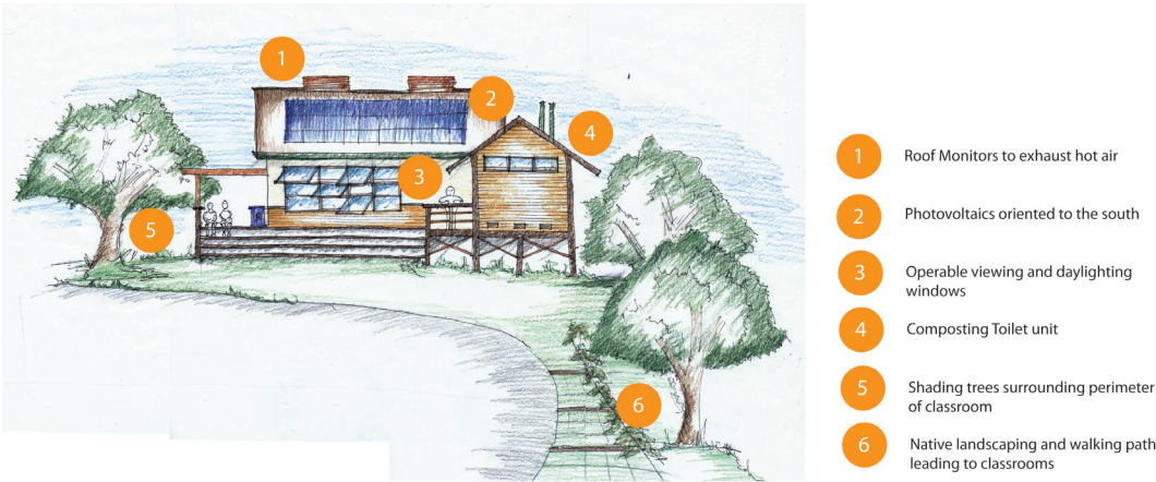
Figure 10.7 Elevation of Classroom Buildings
