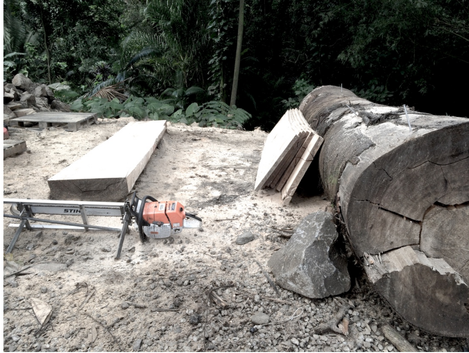
Figure 6.14 Day 4 [January 12, 2016] – Three 1.5” slabs milled
