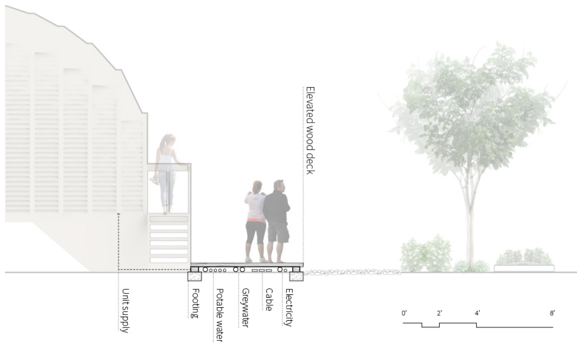
Figure 5.4 Elevated pathway system
