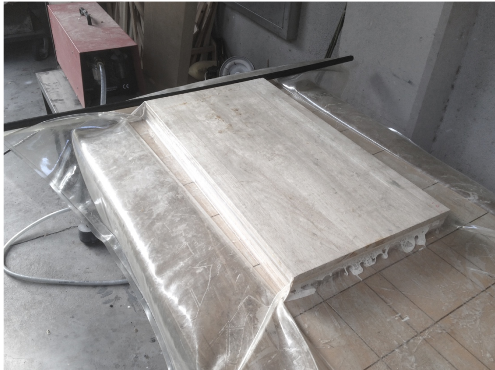
Figure 6.27 Vacuum pressure gluing CLT layers
