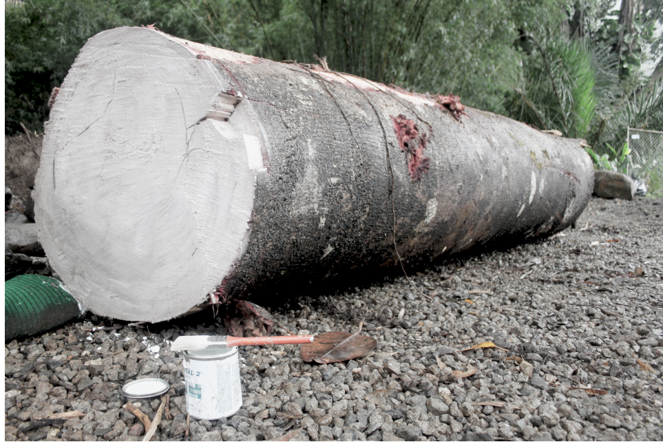
Figure 6.8 Ends coated with Anchorseal green wood sealer
