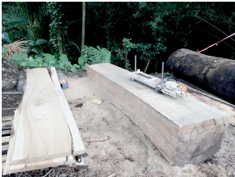
Figure 6.11 Day 2 [December 19, 2015] – Three 2” slabs milled
