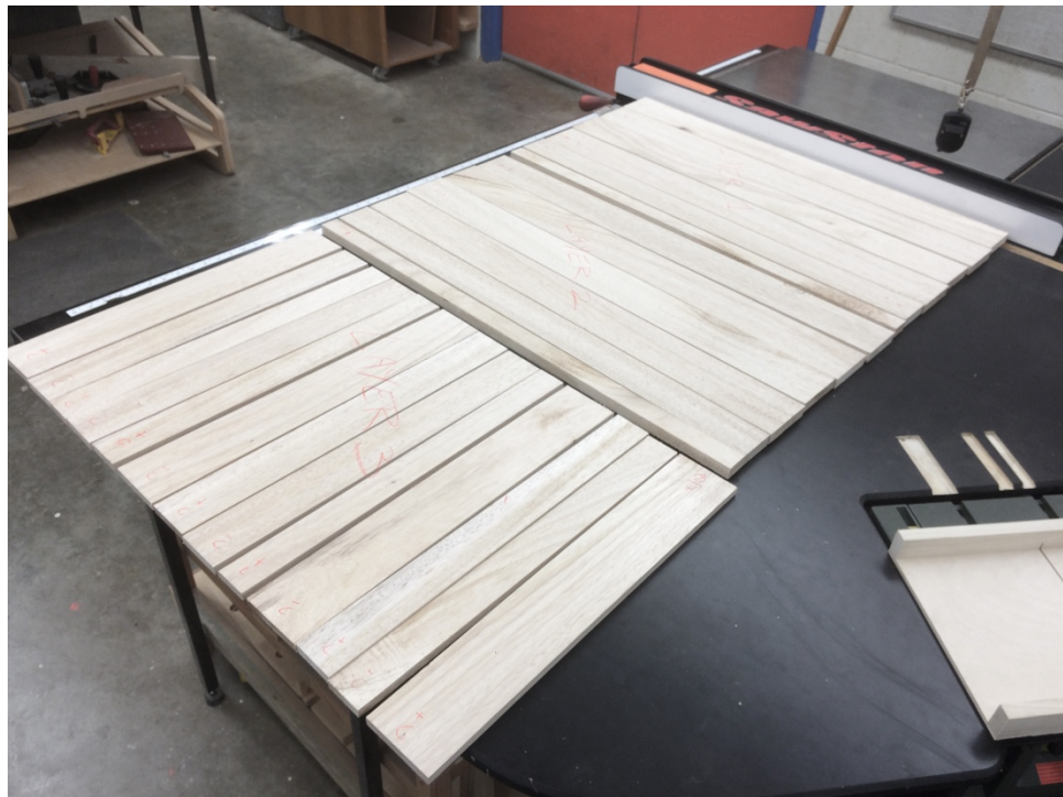
Figure 6.25 Setting up boards for gluing
