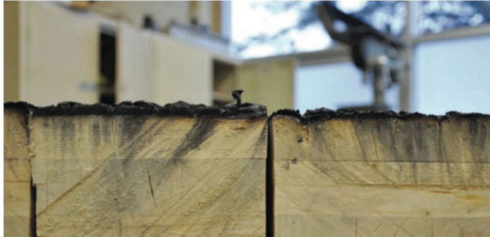
Figure 3.2 CLT testing for fire resistance
