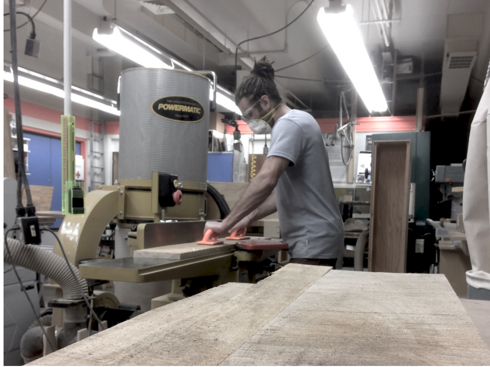
Figure 6.24 Running boards through jointer
