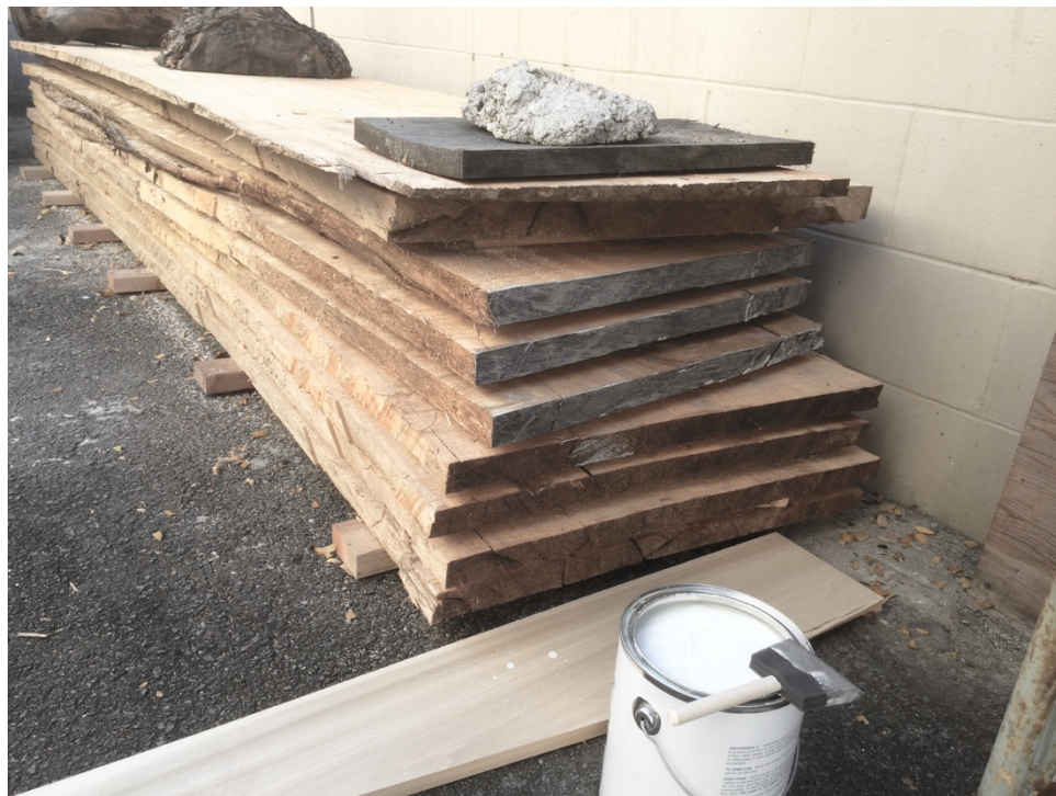
Figure 6.17 Day 5 [January 14, 2016] – Ends coated with Anchorseal
