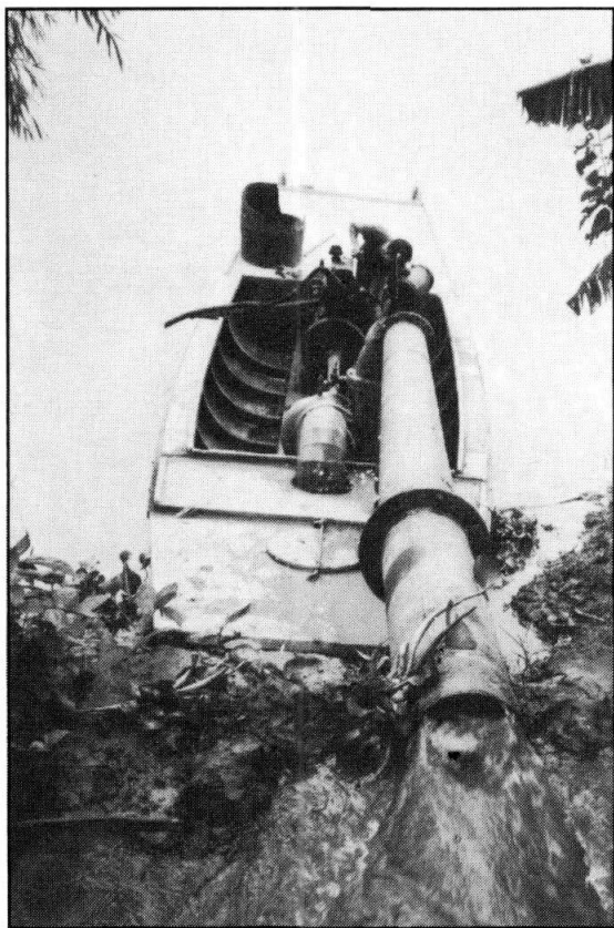
Plate 12. Boat pump, which provides an emergency backup to the pumping stations along the Thong Nhat Canal.
