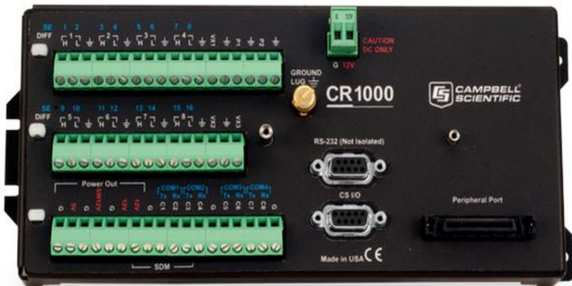
Figure 79 CR1000 Datalogger (Campbell Scientific Inc. 2013)
