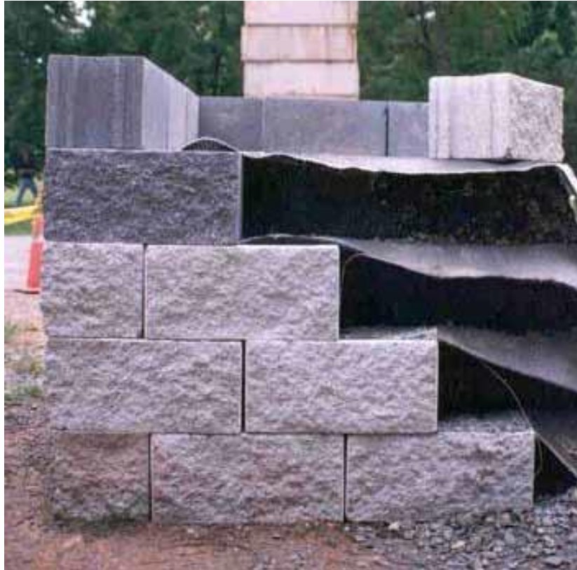
Figure 4 CMU Blocks Commonly Used as Facing for GRS abutments (Adams et al. 2011b)
