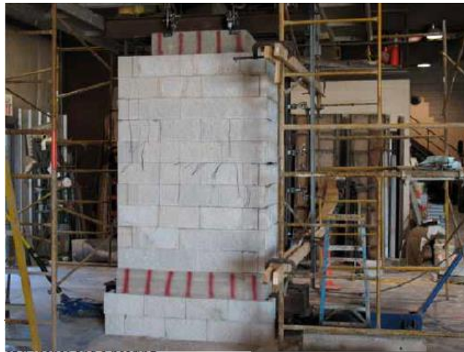
Figure 9 Photograph of a GRS Performance Test Before Loading (Adams et al. 2011a).
